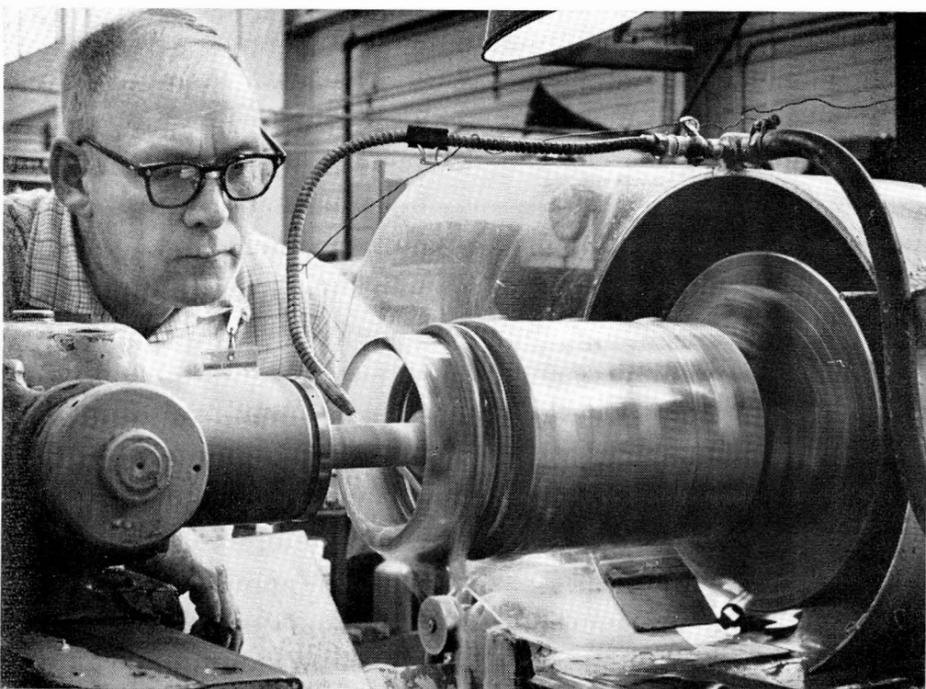
INSIDE DIMENSION of a glass cylinder is ground by Ray Negus. The liquid is a water soluble oil which cools the piece during the grinding operation.
