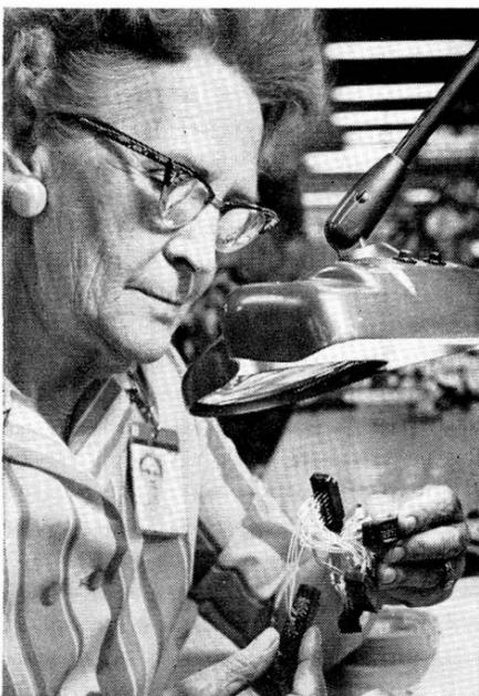
**WIRING HARNESS** is assembled by Mary Kelley. In addition to making cables, the Section assembles printed circuit boards and fabricates wire harnesses for junction boxes. The work is usually one-of-a-kind prototype assembly and requires painstaking care.
