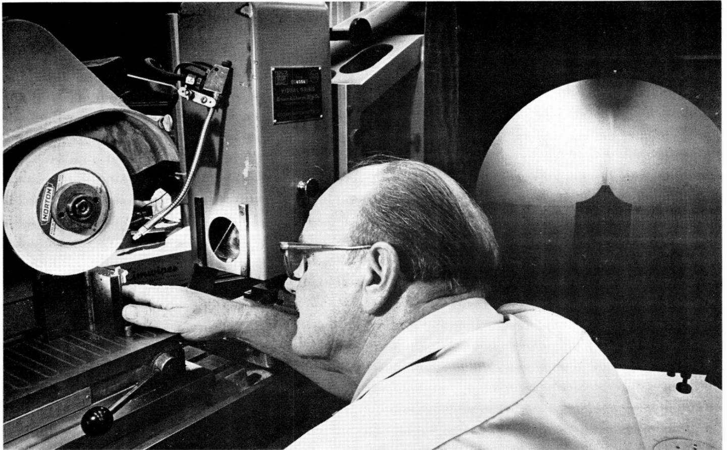
BUCK BABER grinds a concave curve in a small tool. He checks accuracy of the curve by the enlarged image on the optical comparator, right.
