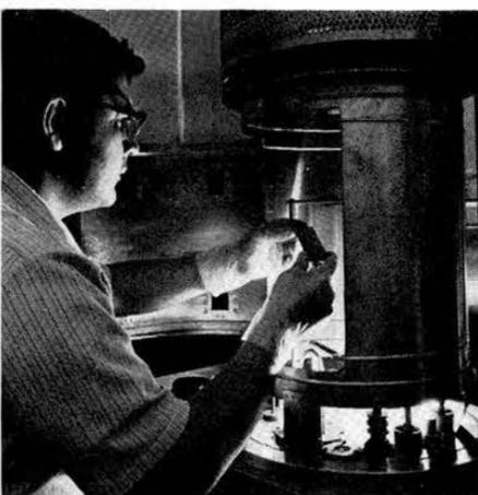
ROBERT MARTINEZ prepares to evaporate aluminum using a vacuum bell jar in the Physical Electronics Laboratory.
