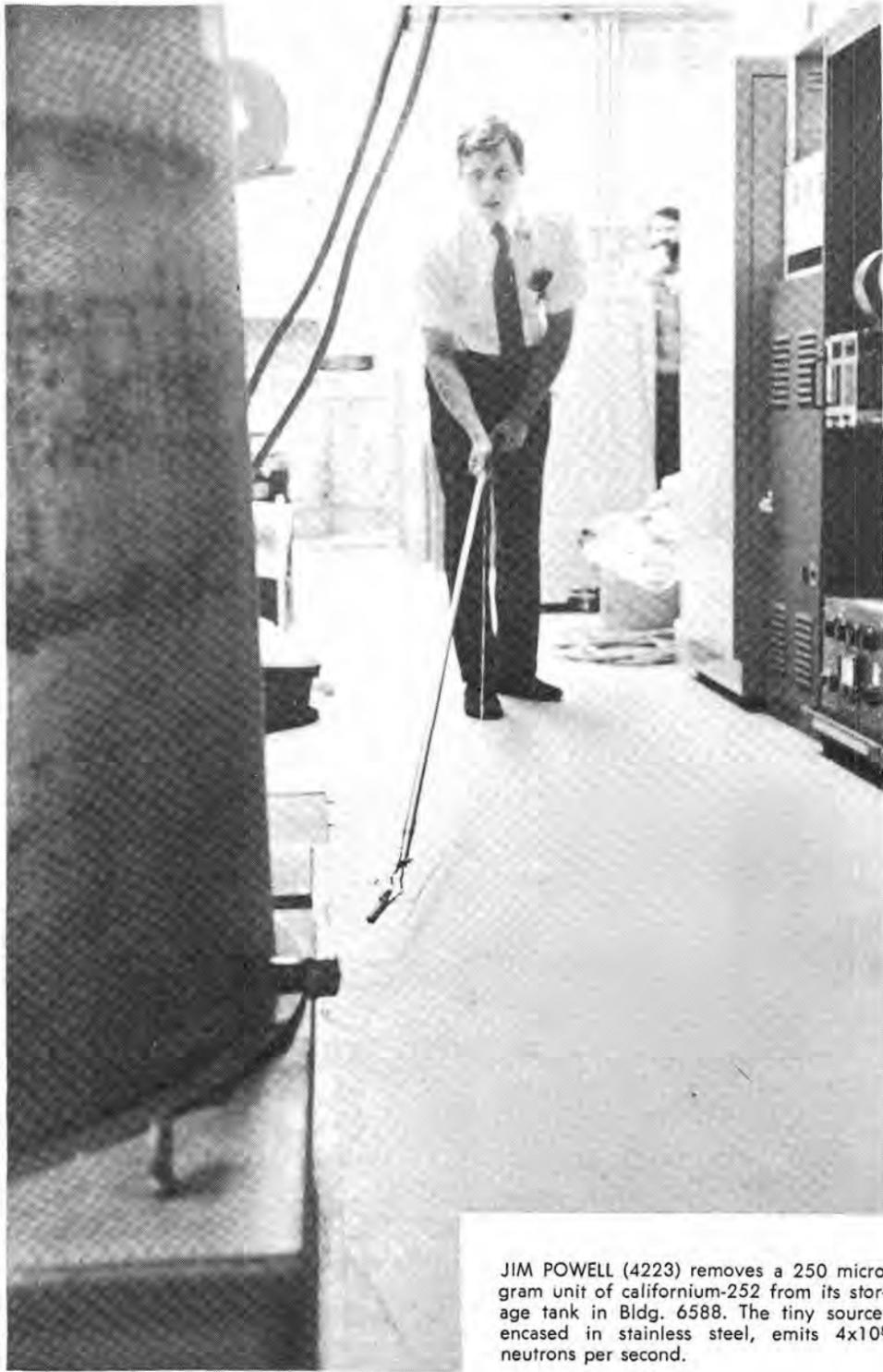
JIM POWELL (4223) removes a 250 microgram unit of californium-252 from its storage tank in Bldg. 6588. The tiny source, encased in stainless steel, emits  $4 \times 10^8$  neutrons per second.
