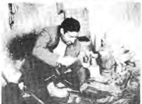
TO MAKE A STEEL FILE, Iranian bazaar style, you need a big toe to hold the metal a steady hand to make the ridges 1/32nd of an inch apart, and a charcoal fire and bucket of water for tempering purposes.
