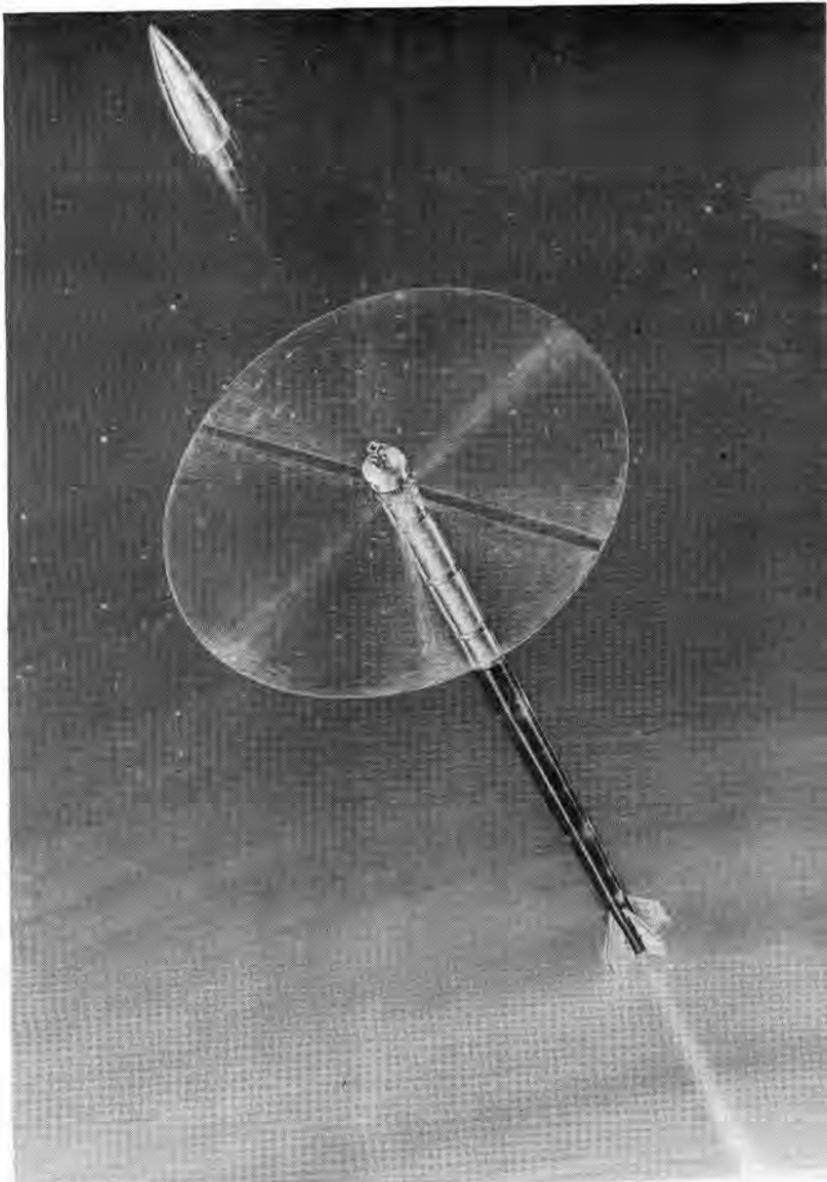
SANDIA-INSTRUMENTED Nitehawk rockets will carry Mylar high altitude samplers during forthcoming shots near Fairbanks, Alaska.
