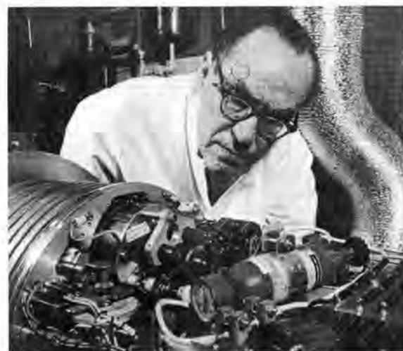
A 400keV Van de Graaff accelerator has been converted to a positive ion source to perform ion implantations. John Smalley (5111) is adjusting the equipment prior to an experiment.
