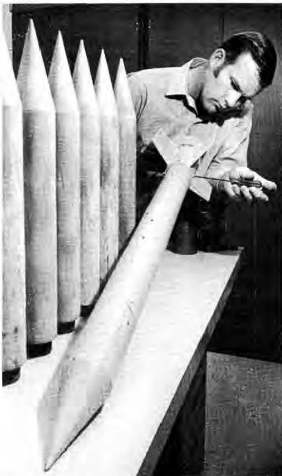
JACK KIKER (9327) assembles Sandia Ice Penetrometer (SIP) planned for use during Coast Guard-sponsored tests in Greenland and northeast Canada in mid-April.
