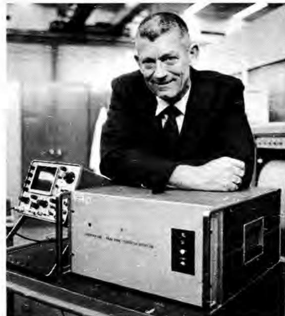
SYSTEM FOR DETECTING airborne particles in a laminar air flow clean room is displayed by inventor Bill Neitzel (9225). Instant read-out is available on a digital counter, a digital recorder, and an audible indicator.
