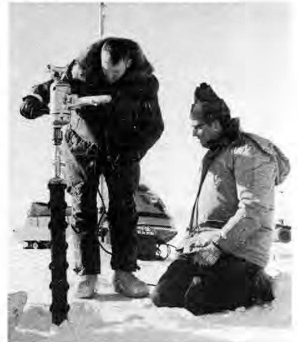
DRILLING a hole in the ice was necessary to get core sample to compare with data obtained by penetrometer. Data thus remotely obtained proved to have high accuracy.
