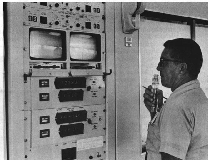
LLOYD YOUNG, using the radar plotting board in the operations room, can control aircraft to plus or minus 25 feet on any given run over the target areas of the range.
