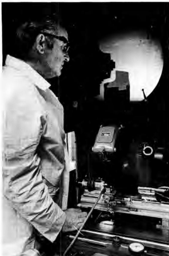
JEWELER'S LATHE connected to shadowgraph is used by Royce Bewely (7142-4) to machine a piece of unfired ceramic to shape depicted on a template. Scope-to-work piece ratio is 20 to 1.
