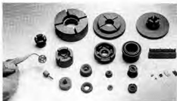
PIECE PARTS of alumina oxide ceramic ( $Al_2O_3$ ), machined in "bisque" state, retain their precise shapes although shrinkage during firing may have been as much as 17 percent.
