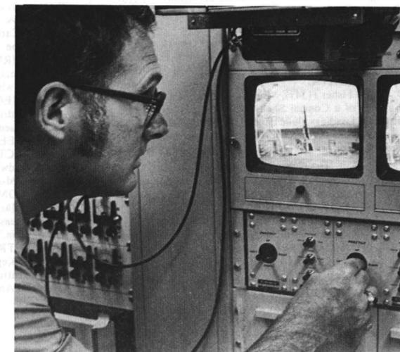
LEO SCULLY, supervisor of Optical Measurements Division, adjusts video monitor prior to firing of a 155mm gun. The big guns see a heavy schedule of tests at the range.
