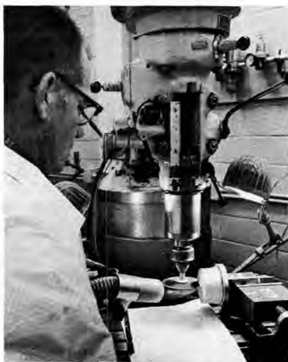
CERAMIC MATERIAL is positioned on a metal holding plate (to relieve strain on soft material) as Charles Ladig (7142-4) operates this mill. Flexible hose connected to a commercial vacuum cleaner keeps machined part clean and prevents inhalation of ceramic dust.
