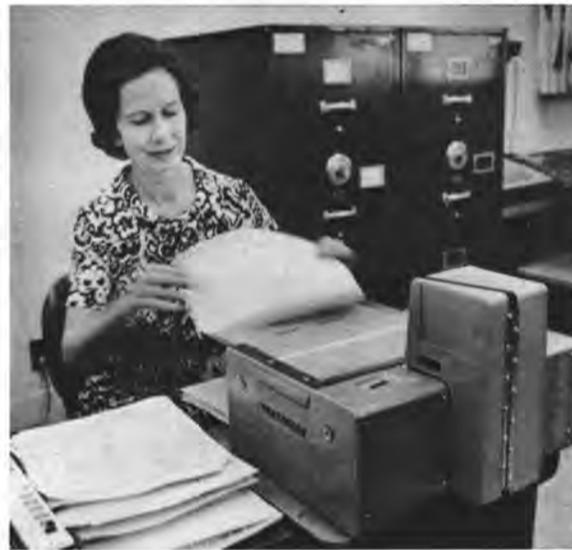
JOHNNIE JOHNSON (9000) demonstrates rapid process of reducing documents to microfilm with a portable automatic unit. The equipment is available by calling Section 7332-1. After microfilming, original documents are destroyed thus reducing need for bulky file cabinets.
