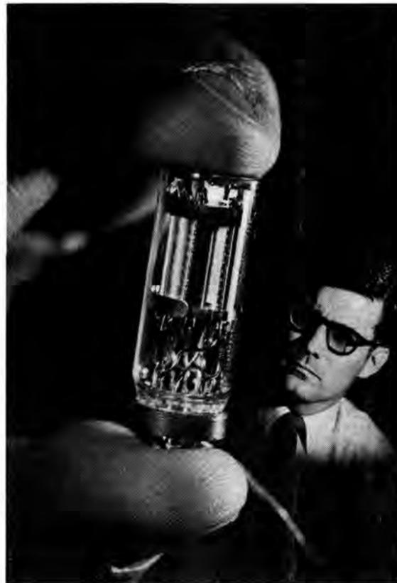
PHOTOMULTIPLIER TUBE held by Joe Vieira (8122) was holographically analyzed in the Photomechanics Lab to detect vibration problems in one of 10 dynodes (components in upper portion of tube).
