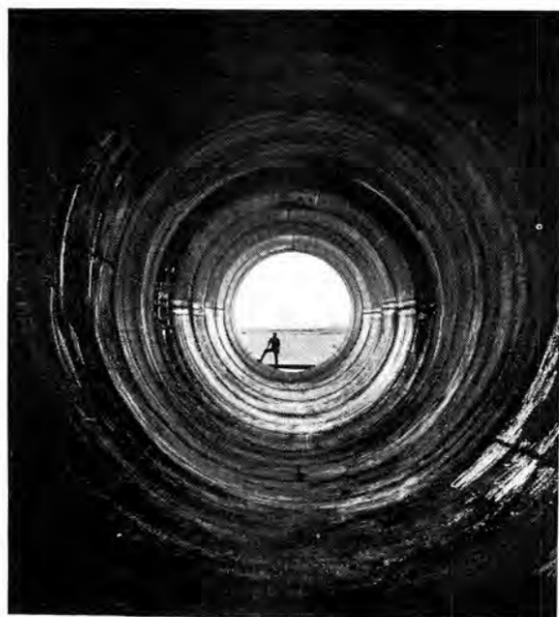
LARGE DIAMETER of shock tunnel test section is graphically illustrated in this interior view. Full-scale test units will be suspended in this section of the tunnel.
