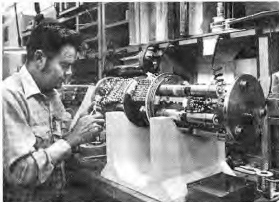
ULTRA-VIOLET PHOTOMETER payload is readied by Jim Reid (9221). The payload will be carried aloft on a Terrier-Tomahawk vehicle.
