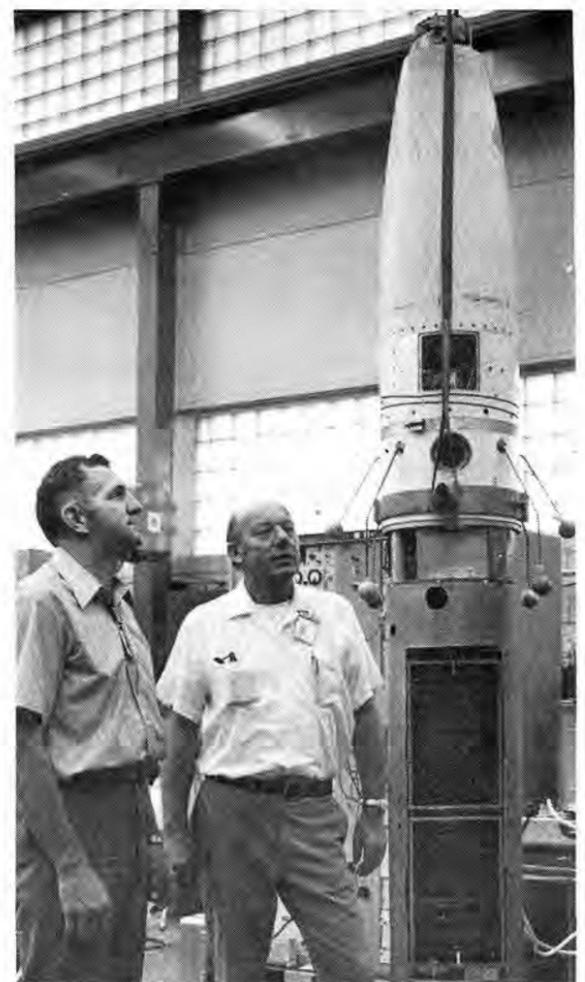
PAYLOAD FOR X-RAY ASTRONOMY EXPERIMENT is examined by Ted Krein and Al Young (both 9221). The experiment package, designed by Lawrence Livermore Laboratory, is located in the bottom half of the payload, and the top half (white cone) contains telemetry and attitude control systems. Terrier-Sandhawk rocket will carry payload to an altitude of about 1.5 million feet during the upcoming series of experiments on Kauai.
