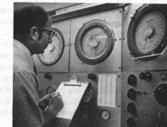
USING THE primary lab's two-pressure humid atmosphere generator, Bill Huff calibrates instruments which measure relative humidity.
