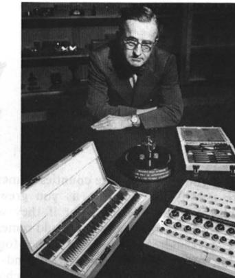
JOE MOODY, an authority on length and mass measurements, displays a few primary standards. The measuring balls are used to compare and calibrate special geometry.
