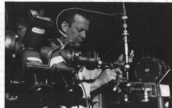
NORM ELLIOTT adjusts the target assembly of a Cockcroft-Walton accelerator used to calibrate pulsed neutron detection standards.
