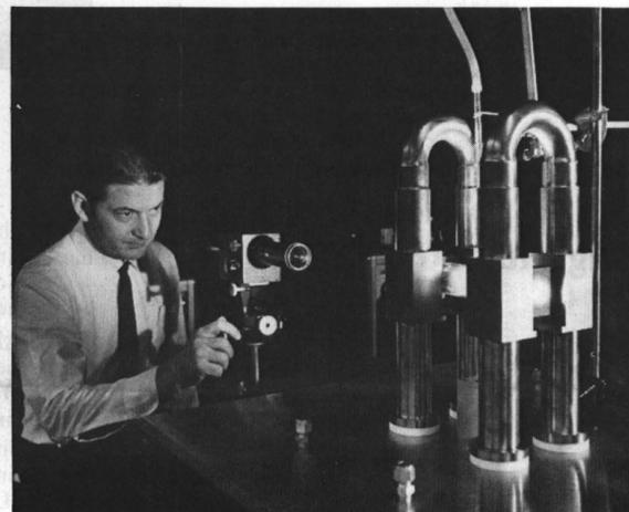
SPECIAL MEASUREMENTS PROJECT is conducted by Bob Foster to calibrate high temperature sensors used in reentry vehicles.
