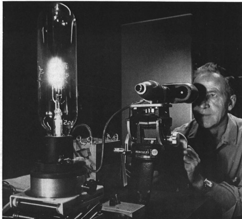
TUNGSTEN LAMP of a known brightness temperature is used by Roy Winter to calibrate an optical pyrometer.
