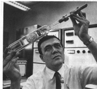
JAY CHAMBERLAIN examines a standard leak — a glass vessel which leaks helium gas at a known rate. The standard is used to calibrate leak detection equipment.
