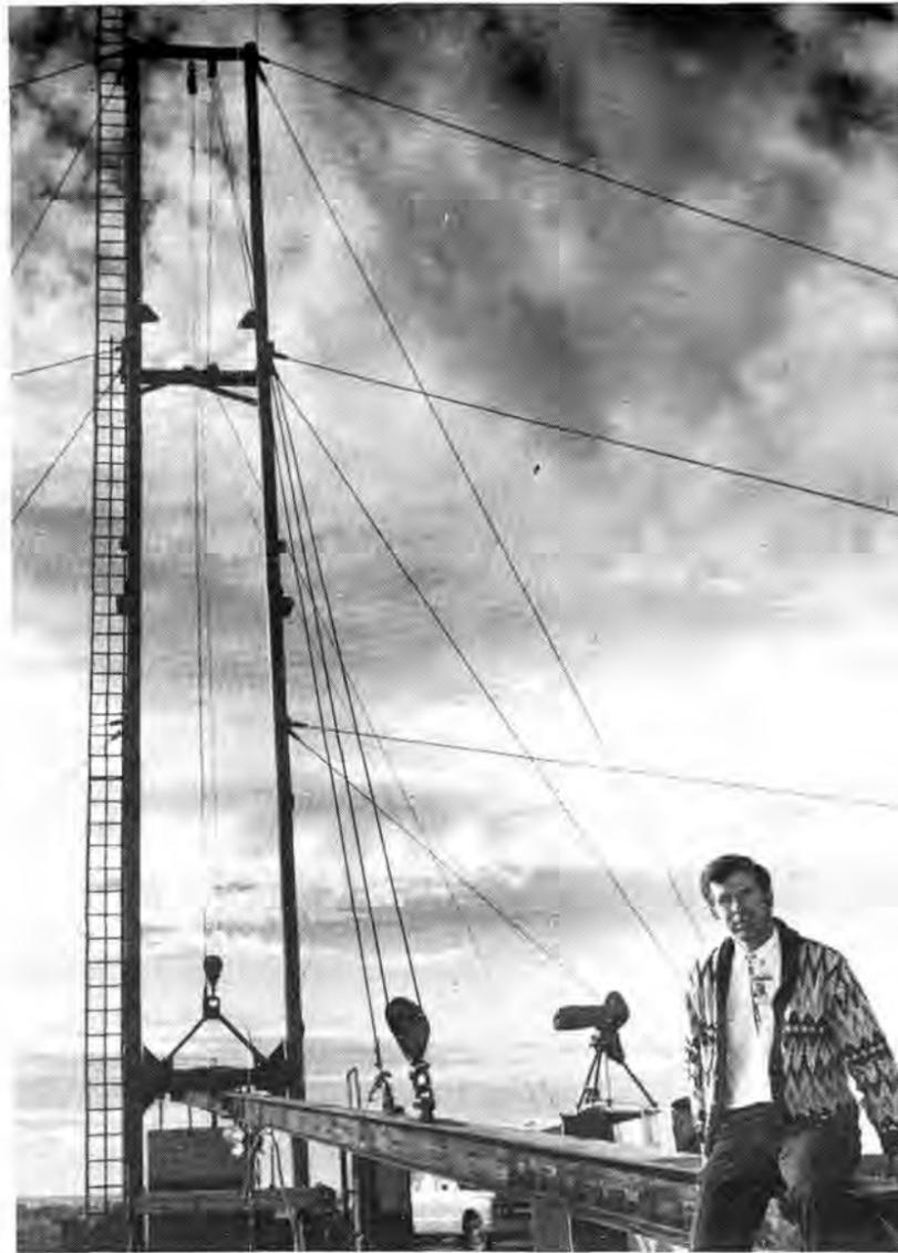
LAUNCHER, ROCKET, Erector Set, is what this arrangement is all about. Marv Timmerman of Tracks and Guns Division 9333 is designer. When end of I-beam Marv is sitting on is elevated, test vehicle suspended under beam is propelled by rockets down into target at whatever angle of impact desired. New facility is located in Area III.
