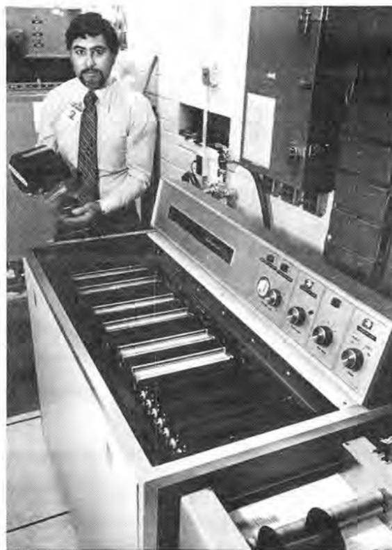
AUTOMATIC FILM PROCESSOR (shown with cover removed) rapidly runs exposed film from the 4460 computer magazine through various chemical solutions to dry reel in foreground. Operator is Joe Tapia (5411).
