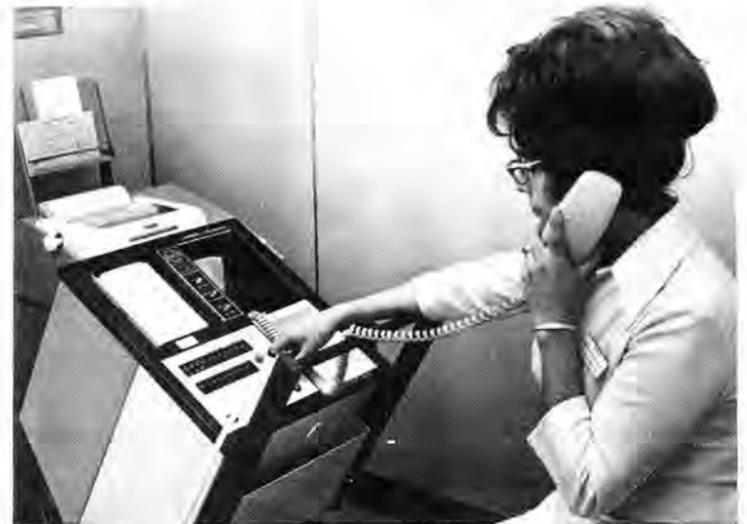
HEART TALKING TO CHICAGO COMPUTER -- Nurse Mary Winter (3302) fixes an electrode to patient's arm (left), then uses phone lines to feed electrocardiogram of patient to Telemed in Chicago (right). The device is a "Patient transmitter" and gives a complete reading on the state of a heart in a few seconds. In addition, a local printout makes it possible for Sandia physicians to check the areas of possible concern identified from the computer feedback.
