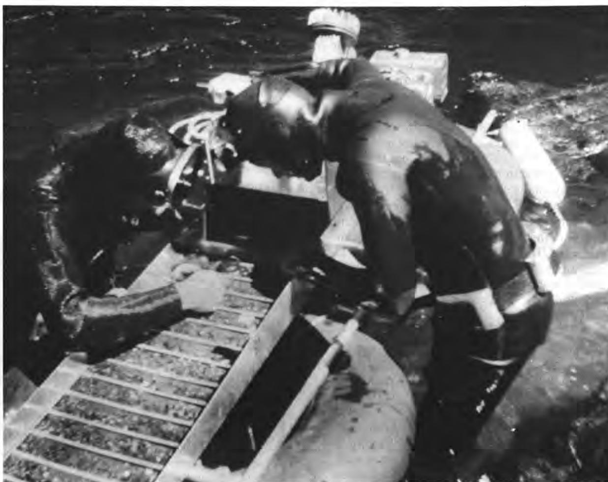
SKIN DIVERS Kirby Hammond (8422), left, and Don Sadler (8421) operate a small portable dredge and sluice box prospecting for gold. Although the portable dredge has its limitations and is used primarily in prospecting, it is more versatile and easier to transport than heavier equipment used in mining operations.
