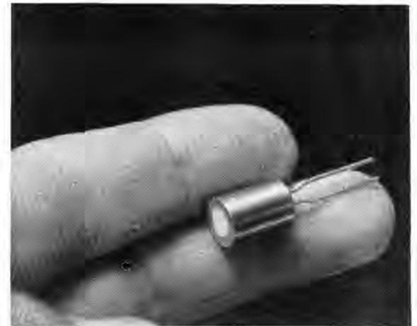
HIGH TEMPERATURE resistant exploding bridge wire detonator invented by Bill Leslie (1915).
