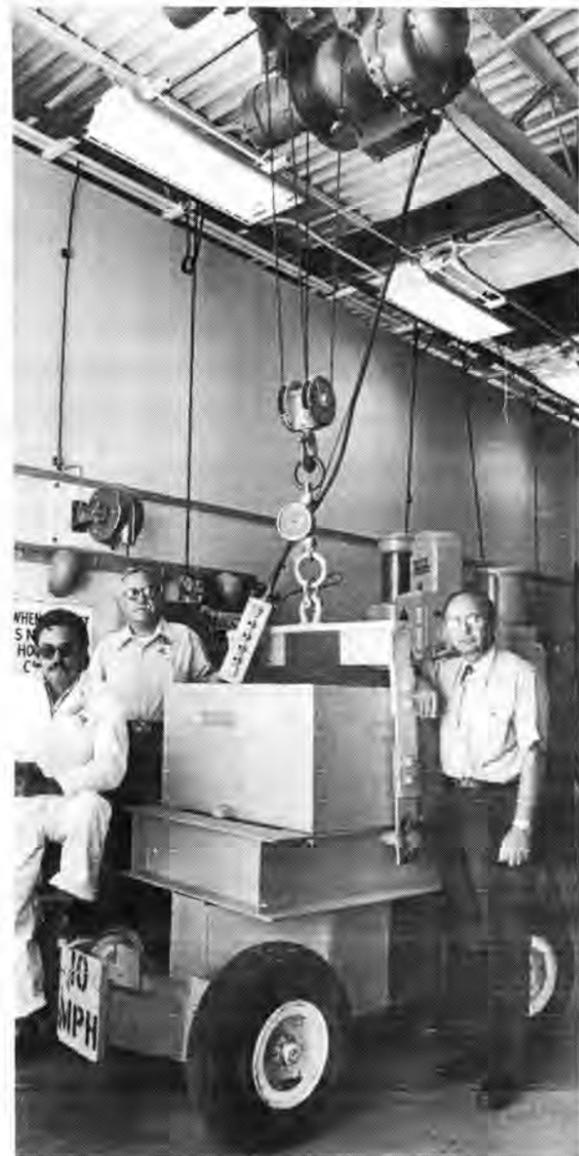
LEAD FILLED TRAILER weighing 18,750 lbs. is saving Sandia time and money in testing hoists in Area III. The trailer replaces large concrete blocks and several pieces of heavy equipment previously used. Idea was conceived by Marv Austin, right. Tom Sanchez, left, designed the trailer and helped Pat Lerma build it from salvaged parts.
