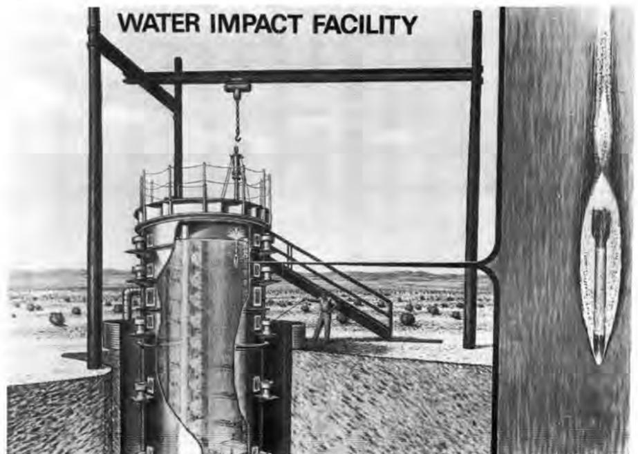
WATER IMPACT FACILITY — A filtration system assures clear water in this 14 by 22-foot tank. Atmospheric pressure and density above the water can be controlled. Air guns mounted on the lid propel models into the water at velocities up to 900 fps (600 mph). Ten high-speed cameras look through portholes to record water entry events. Inside, 56 1000-watt lamps provide illumination.
