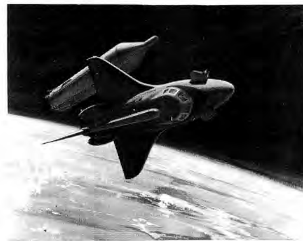
TANK JETTISON — Space shuttle orbiter jettisons external fuel tank shortly after reaching orbital altitude above Earth. The tank, which carries propellants for orbiter's main engines, re-enters atmosphere to impact in preselected ocean area.
