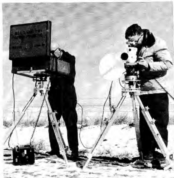
PARC (Position and Release Control) instruments which bring the Beaver onto target and signal release time of test units are operated here by Gordo Miller, left, and Cal Cox.
