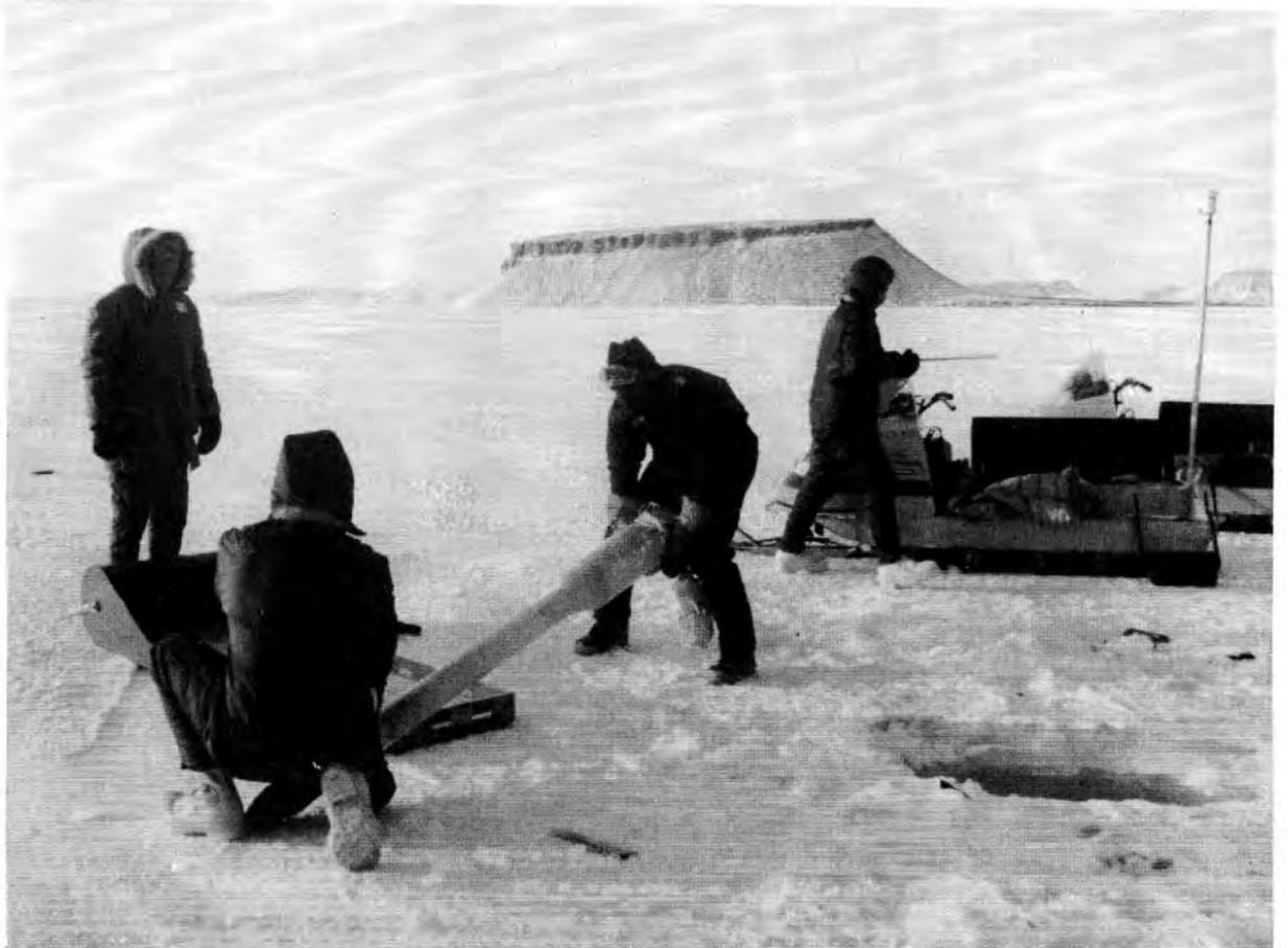
RECOVERY of an ice penetrometer test unit is performed in below zero temperatures. Face masks are a necessary precaution. Sea ice thickness averaged about five feet in this area. Eighteen test units were successfully dropped and recovered.
