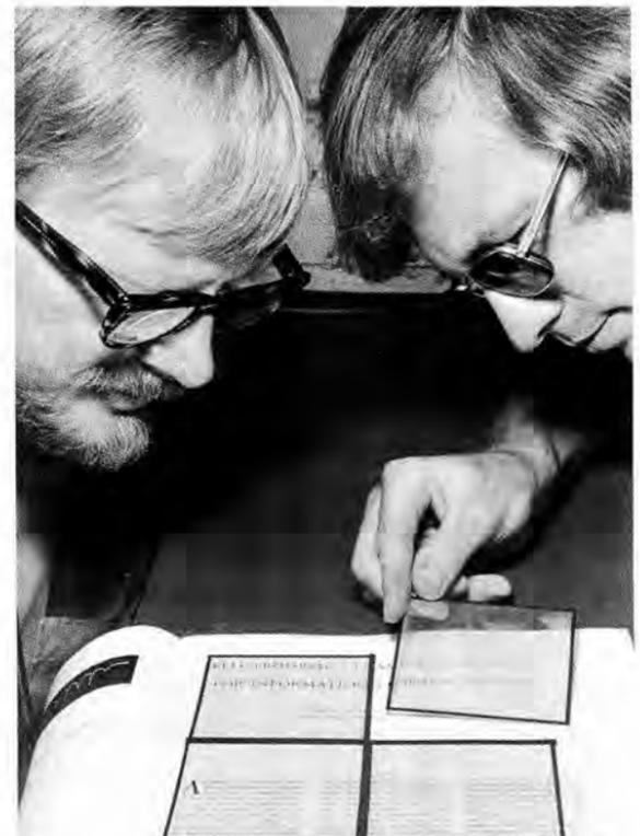
TRANSPARENCY of PLZT material is demonstrated here by Tom Cutchen and Jim Harris (both 2521). The segments will be assembled into an aircraft window together with sensors and circuitry that enable the window to turn opaque so that the aircrew is protected from thermal burn and flashblindness. They were fabricated in Sandia's Ceramics Shop (7122-1) under the direction of Gary Snow (2521) and Bob Dungan (7120).
