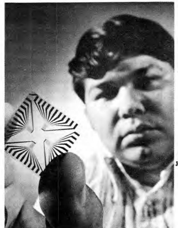
GEORGE LAGUNA (2521) displays prototype of a ceramic light gate. An array of 256 of these tiny shutters will serve as an information input device — page composer — for an optical (holographic) computer memory.
