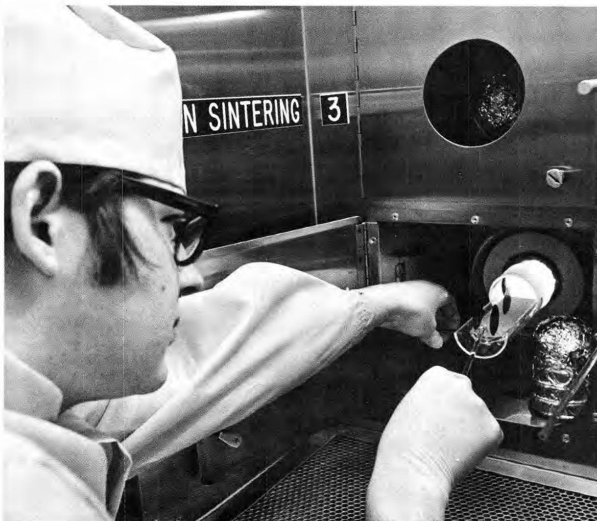
INTO THE FURNACE goes a boatload of semiconductor wafers. Doug Weaver does the launching. The new lab includes the most recent equipment and techniques for semiconductor fabrication.
