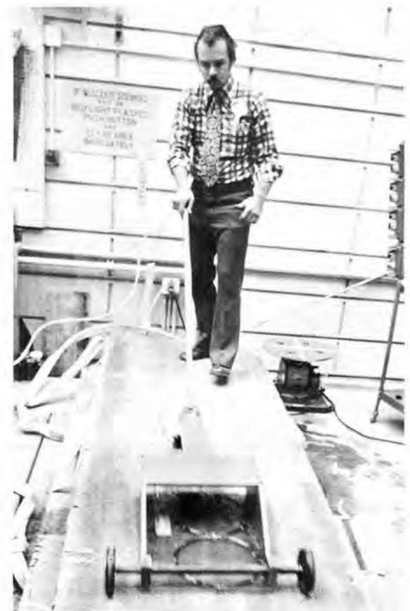
JIM BUSHNELL (9532) checks out twin-coil magnetic detector on a 3000-lb. sample of highway concrete. The device helped resolve a controversy about the amount of rebar in a new stretch of I-25.
