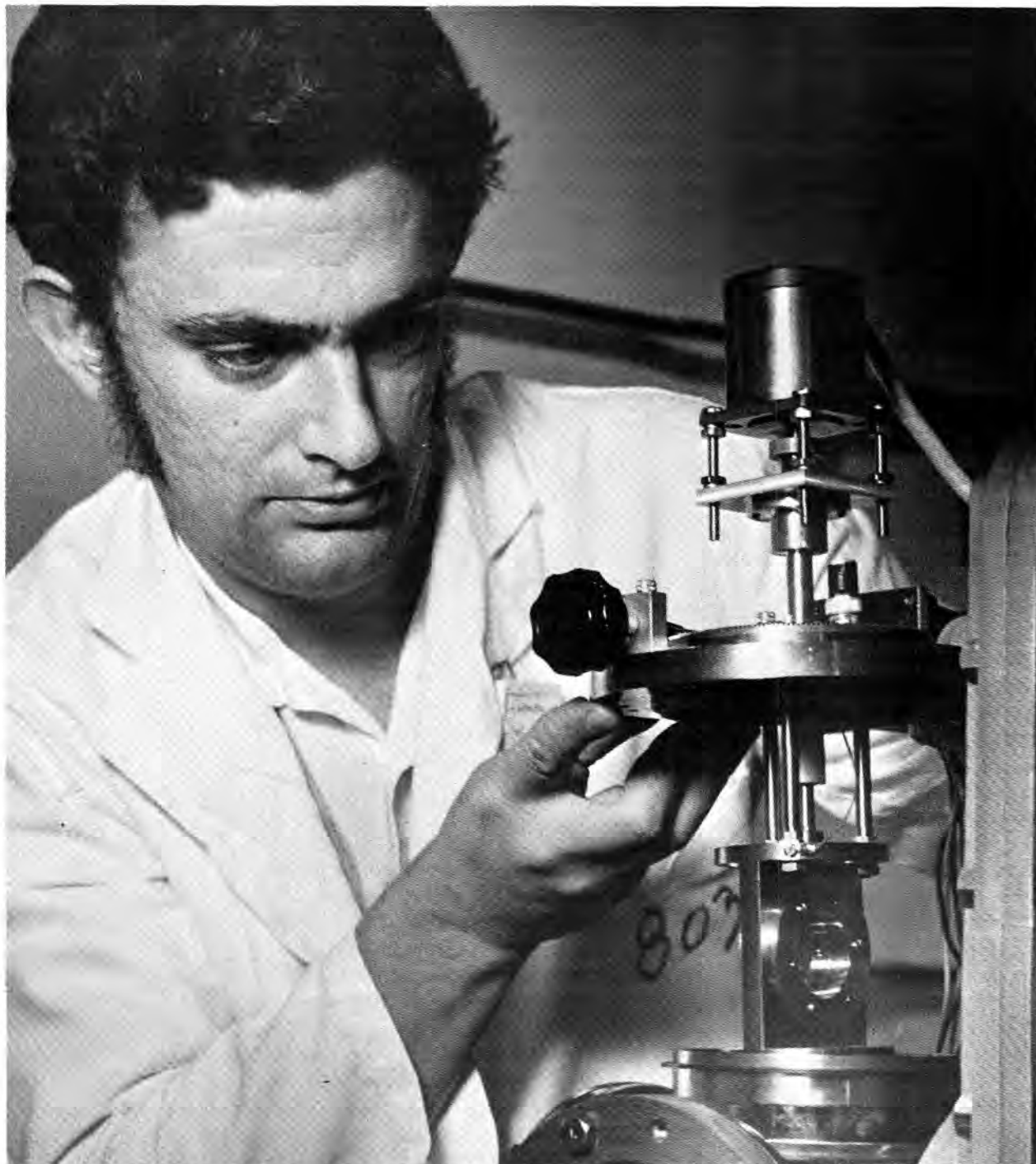
A GONIOMETER, containing a sample to be implanted with ions, is lowered into the working end of the Bldg. 803 accelerator by Jim Borders (5111). The device permits almost infinite adjustment of the angle of exposure. The sample itself is inside the cylinder to the right of the "803" on Jim's coveralls.
