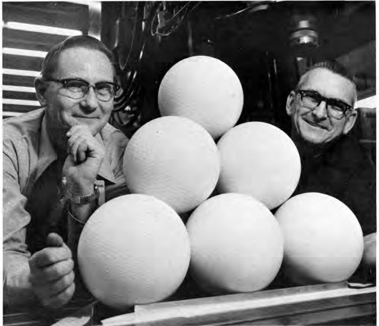
**BOWLING BALLS** they're not. They're 8" polyethylene spheres which will be criticality monitors near our nuclear reactors. Two kinds of dosimeters will fit into the small hole in each, with the sphere serving as neutron thermalizer. Dan Thompson (3313) has project responsibilities, but the precision machining was done by Keith Gawith (left) and his trainee, Jake Young (both 7146).
