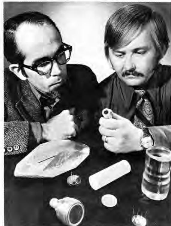
Bob Graham (left) and Ron Jacobson (both 5132) examine the new lithium-niobate gauge they developed to measure shock wave pressures up to 250,000 pounds per square inch. Shown in the foreground are (l to r) quartz, sapphire and lithium niobate crystals which Bob and his collaborators at Sandia have used to make three different gauges. The gauges utilize the special properties of crystals to measure shock wave pressure.
