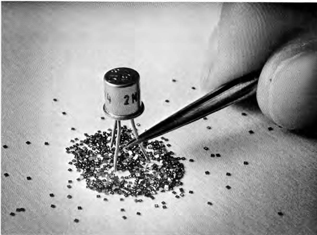
ONE METHOD of miniaturizing components is to eliminate bulky containers. Here a standard transistor bestrides several hundred transistor chips. A single chip in a hybrid circuit typically performs the same function as the large transistor in the container.
