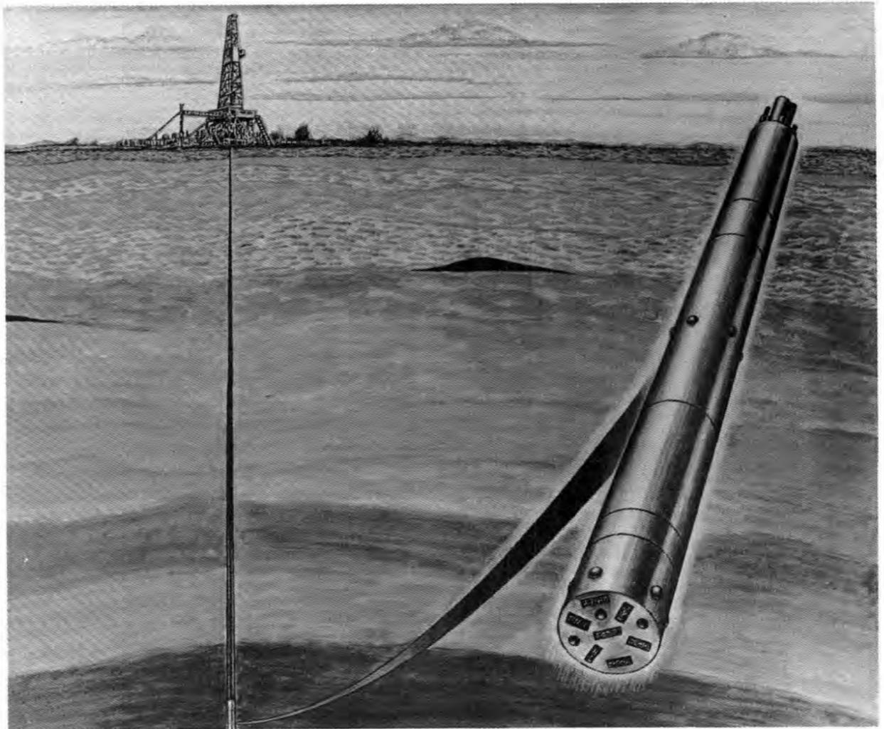
ARTIST'S SKETCH shows the proposed Sandia shock generator at the end of an oil well drill stem. Wireless detonators are at the bottom of the 10-ft. shock generator unit.
