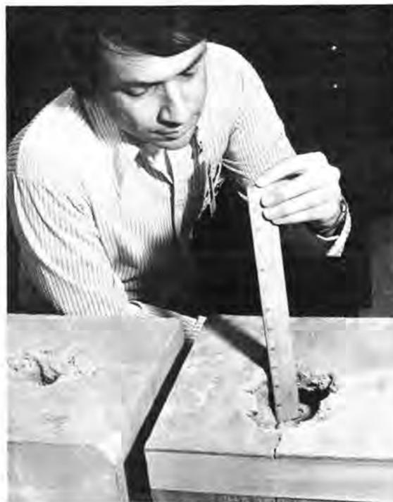
HOLES punched in solid concrete blocks in the laboratory by the drilling head average five inches in diameter, about three inches deep. Robert Silva (5724) displays a couple of the test blocks.
