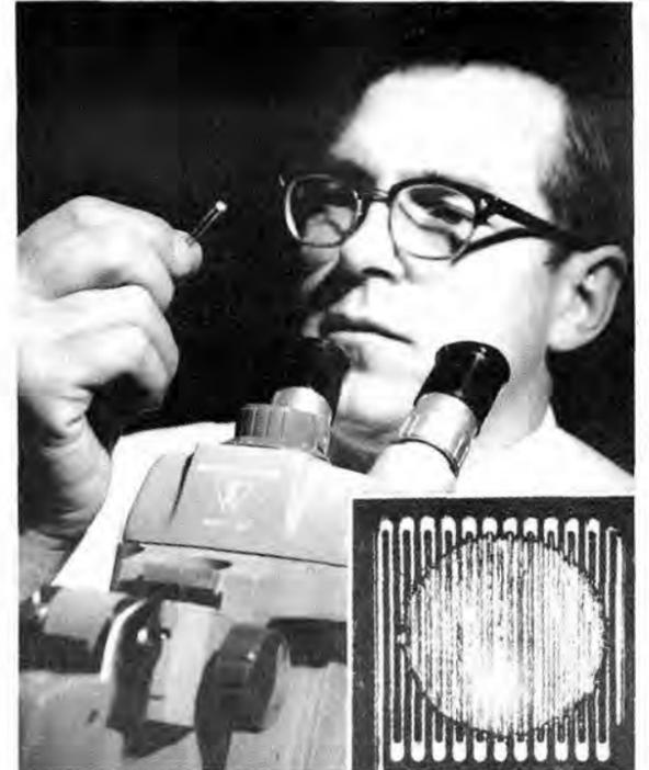
VERN BARR (8342) checks masking before manganin foil gage is plated to modify its physical definition. Inset shows gage grid after plating.
