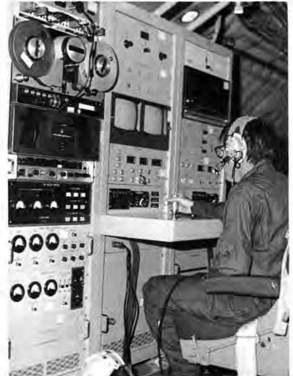
AT THE ALOTS console inside the aircraft is Al Watts (1255). Operator locates a target on one of the two TV screens above him and locks the tracking cameras on it. Just before impact he starts the cine camera which records the event.
