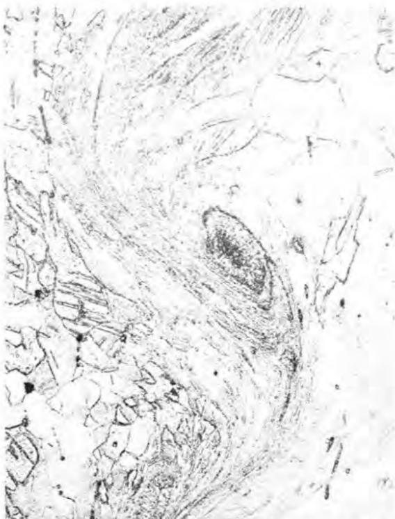
PHOTOMICROGRAPH shows bond region (at 400X magnification) between copper plates produced by impact welding technique.
