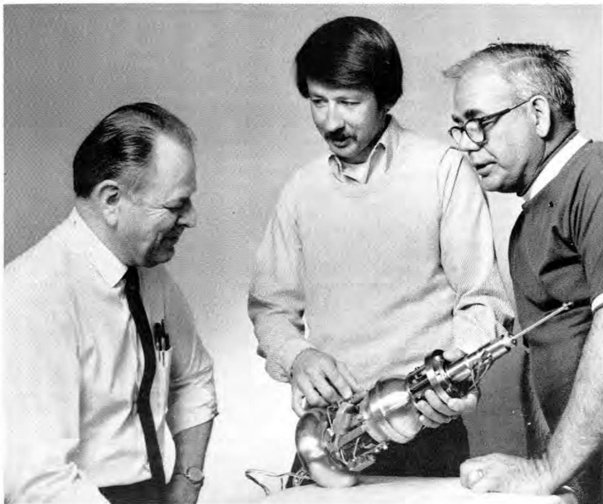
SLL-DEVELOPED EXPULSION SYSTEM and instrumentation recovered from recent rain erosion flight tests of transpiration cooled nosetips (TCNT) are examined by (from left) Mac Spivey, Bill Wilson and Roy Tackett (all 8362).
