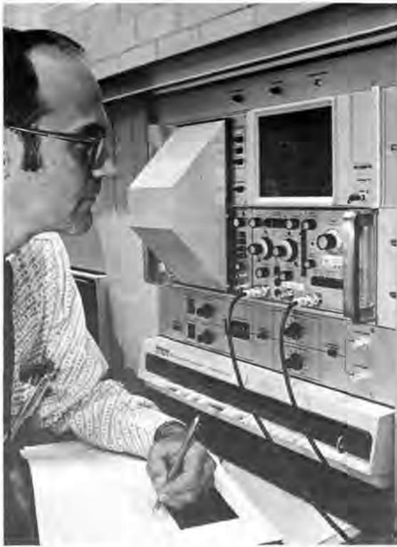
LABORATORY MODEL of the vidicon digitizer is checked by Thomas Evans (2342), a co-developer of the system. From top to bottom are oscilloscope, digitizer and computer.
