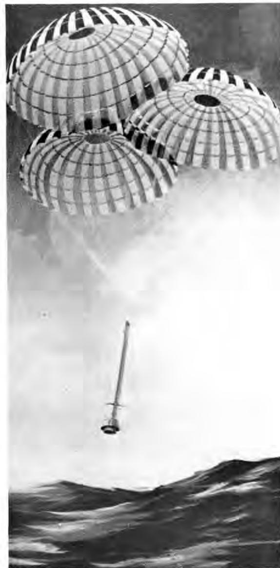
DRAWING shows one of the booster rockets of the space shuttle with full deployment of the main parachute array. Sandia is aiding NASA with the design and development of the recovery system for space shuttle booster rocket.
