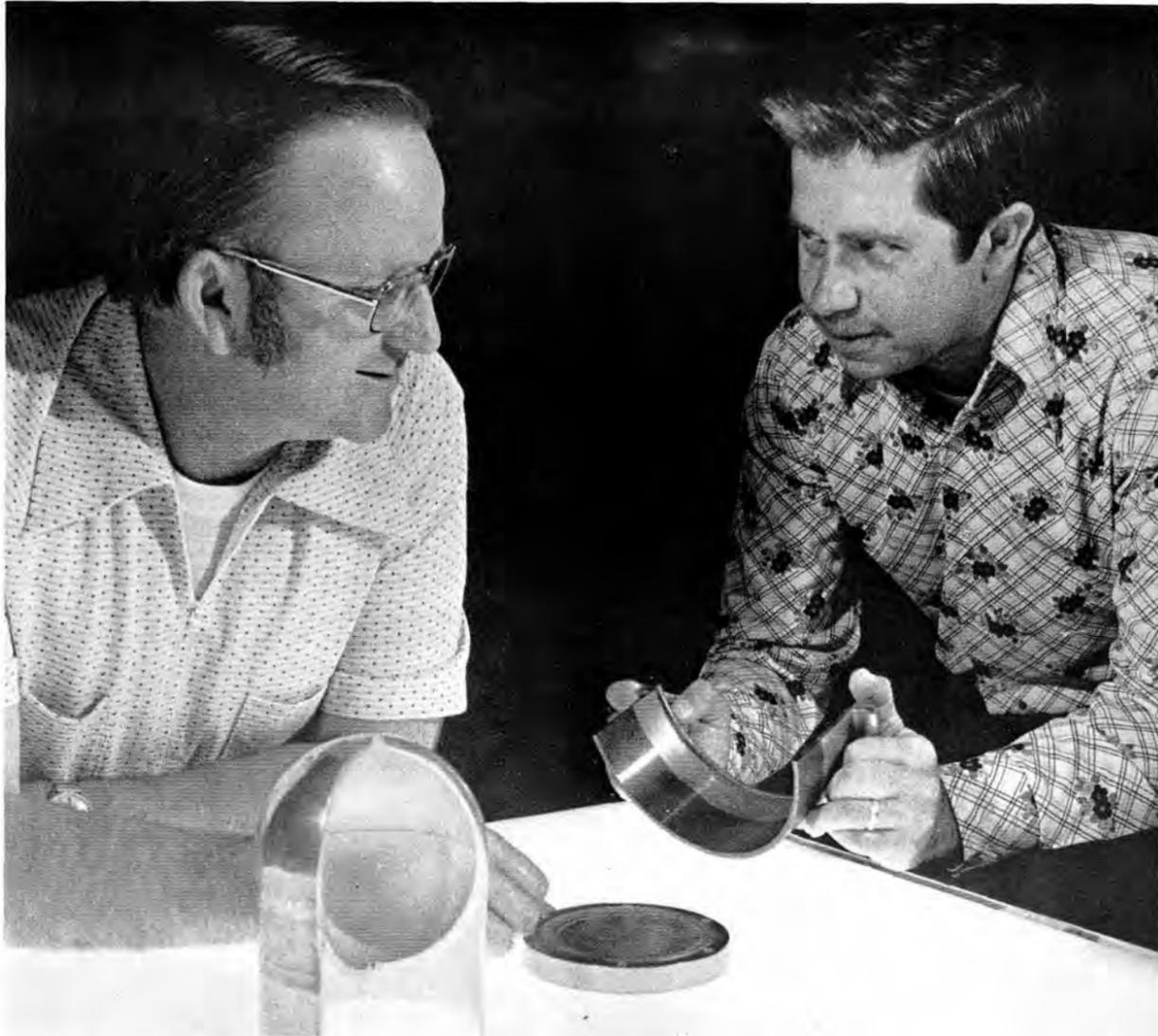
COMPULSIVE JOINERS— Rudy Johnson, left, and Jack Dini (both 8312) examine an electrochemically joined specimen of stainless steel and uranium. The two metallurgists have developed process for joining of materials previously not joinable.
