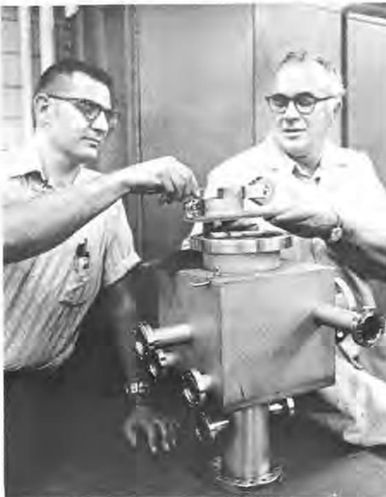
*IT'S METRIC* — first all metric job out of the machine shop was completed by Jim Myers (left) and Joe Shelby (both 3644-2). The unit, a vacuum chamber with a turret mechanism to hold samples (on top)/(held by Joe), "proves that even a guy with 36 years of working with inches can adjust to millimetres," says Joe. Adds Jim, "We're getting more metric tools and converting more machines all the time." The chamber was constructed for Dal Jensen (2413) with drawings by Johnny Baca (9611).
