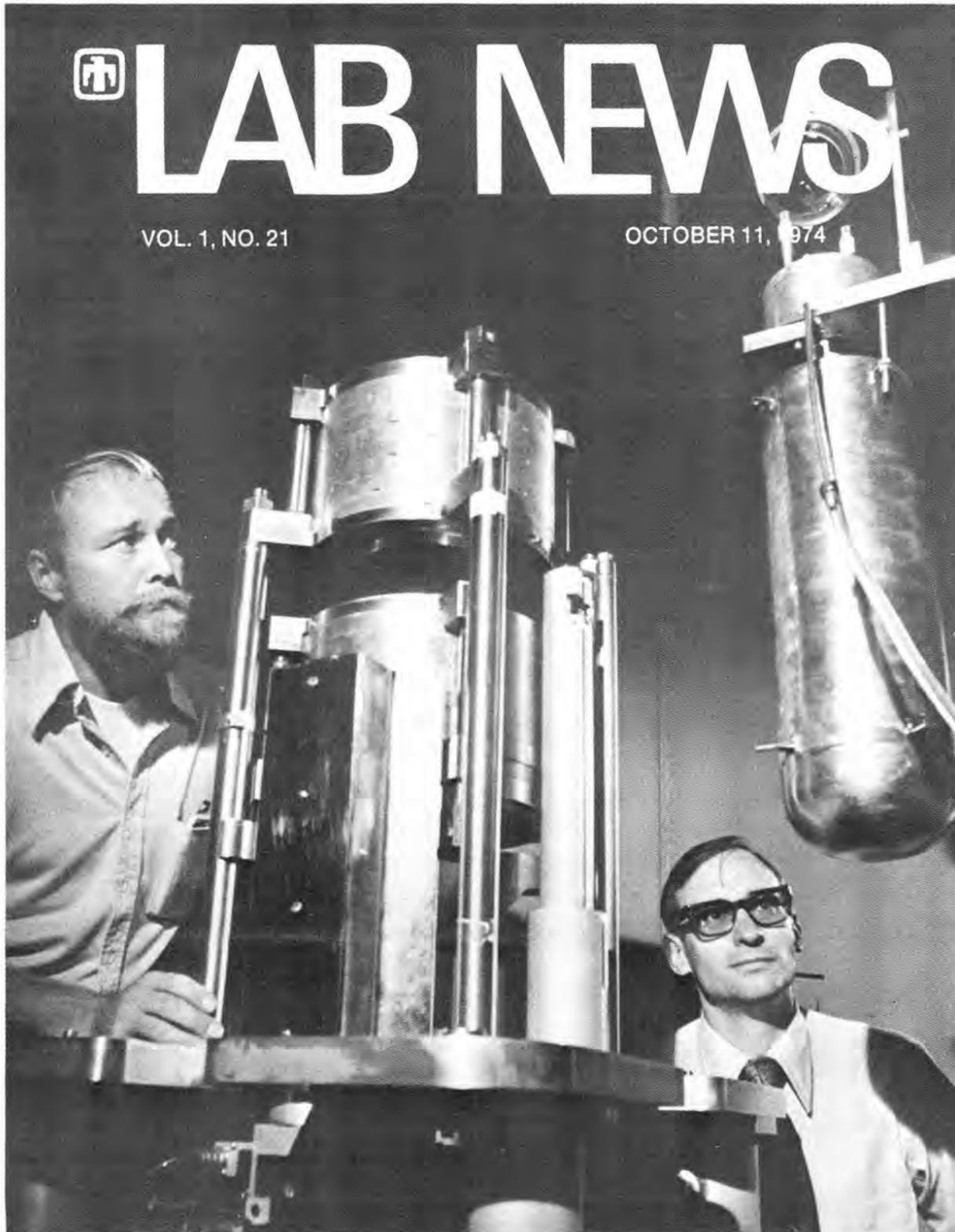
PRINCIPAL INVESTIGATORS on the reactor-pumped CO laser, Phil Tollefsrud, left, and Dave McArthur of Dep't. 5220 are shown with the laser, upper right, and a mockup of the SPR III, Sandia's newest pulsed reactor. This is believed to be the first laser produced by pumping with fission products.
