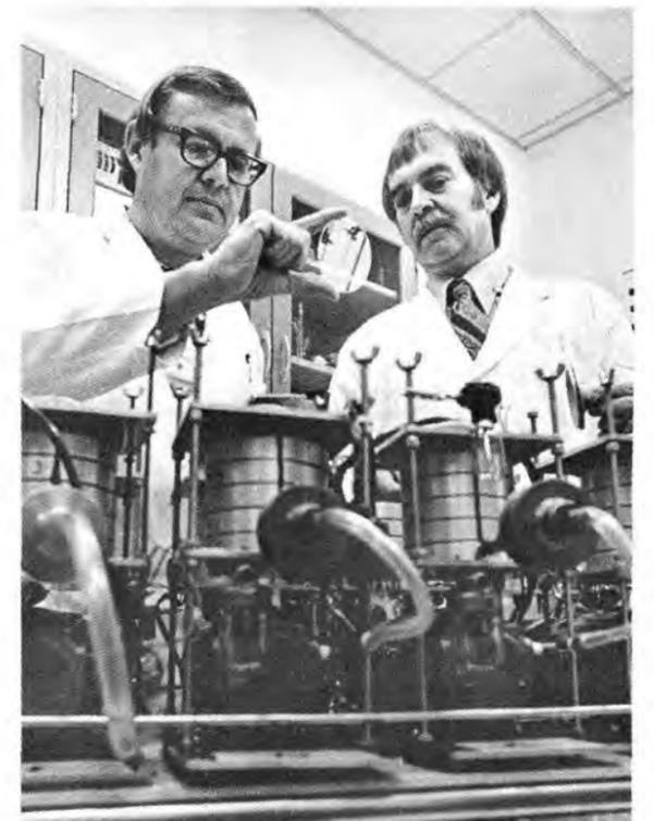
THE ANDERSON AIR SAMPLER separates dust by particle size and deposits the particles on glass disc. Charles and Lial examine one of the discs before insertion into the sampler; later the deposits will be analyzed to determine if toxic dusts are present.
