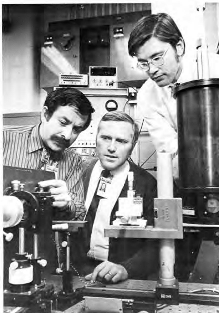
KEN TOURYAN (5640, left) adjusts the entrance slit on a tunable diode laser as Colin Hackett and Dave Smith (both 5642) look on. The laser would be a primary analytical tool of a stratospheric measurement program.
