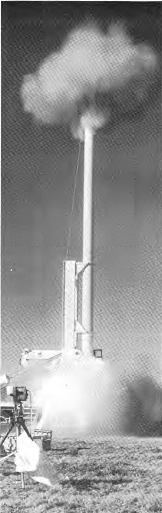
NEW DOWN-FIRING GUN recently underwent a series of test firings near Edgewood. The gun is used to fire projectiles into the ground as part of the Labs' continuing terradynamics program.
