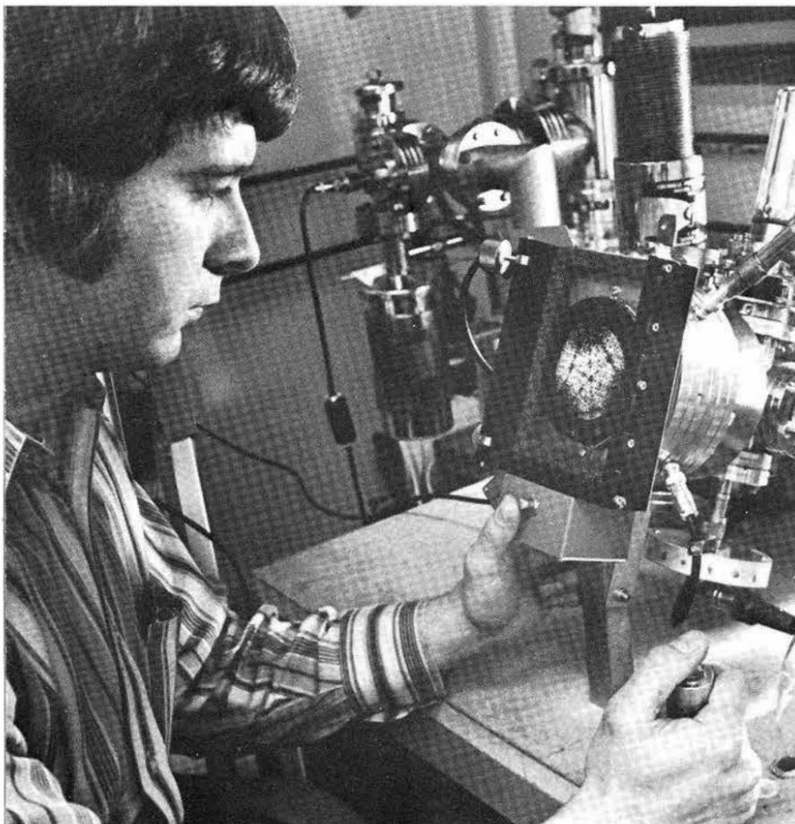
JOHN PANITZ (5114) looks at helium on the first atomic layer of a solid surface through the viewer of a unique new instrument he invented. Called an imaging field desorption mass spectrometer, it was recently patented by ERDA. Bob Crozier (3646), Foster Tennant (3621) and Jim Taylor (3623) contributed significantly to fabrication of the instrument in the Sandia shops.
