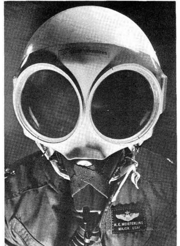
HOW'D you like to meet this character on a dark night? It's not likely unless you take up flying with the Air Force. He's wearing Sandia's thermal and flash protection goggles, whose lenses are made of PLZT ceramic. Goggles prevent blindness from flash of nuclear burst.
