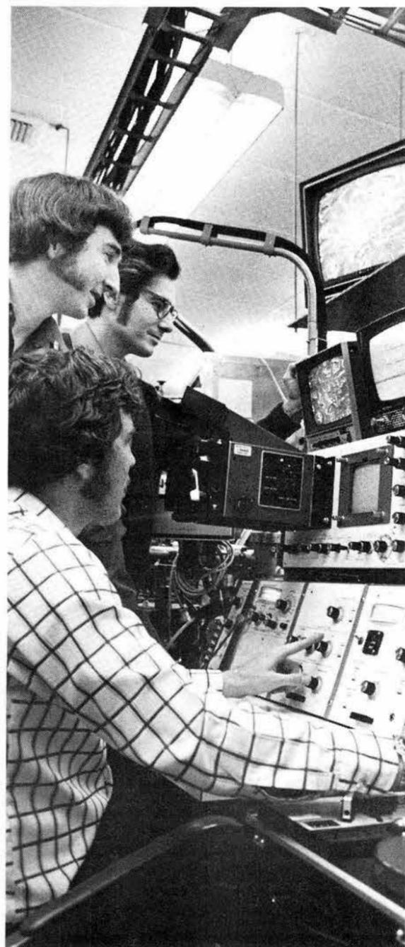
DETAILS OF DEVASTATION on a molecular level are seen when a material sample is subjected to CTR environment. Video system is connected to a scanning electron microscope focused on the target area of a 450 KeV positive ion accelerator. Researcher George Thomas (8334), upper right, Dan Morse (8334) and operator Les Brown (8313) conduct the experiment.
