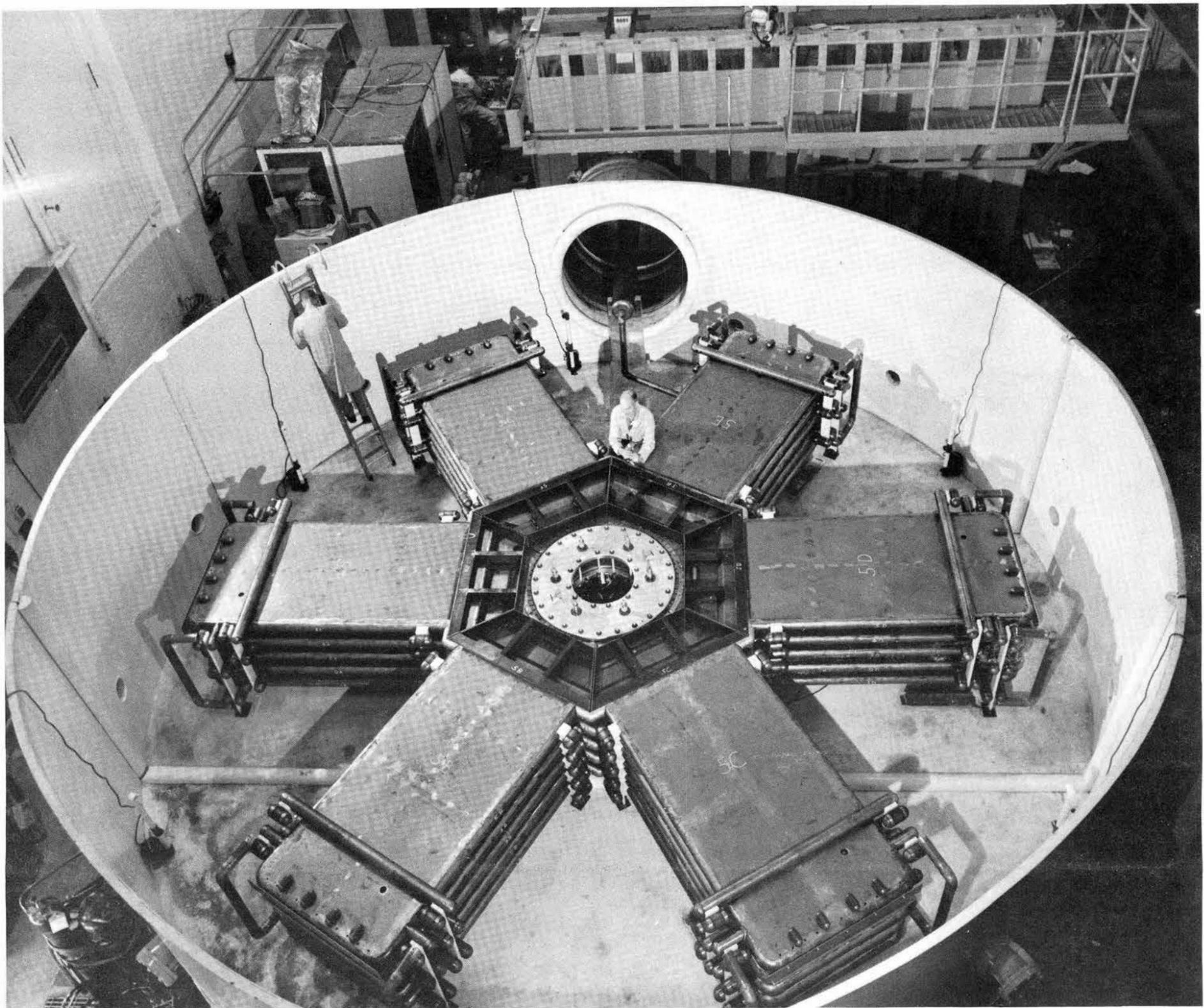
MEET PROTO 1, Sandia's newest and largest electron accelerator. With it, Plasma and Electron Beam Physics Research Department 5240 will study the feasibility of using electron beam fusion to generate electricity. Proto 1 will develop 2 to 2-1/2 trillion watts during its 24 billionths of a second pulse. If experiments at those levels succeed, a second accelerator will be built. It would be capable of fusing
