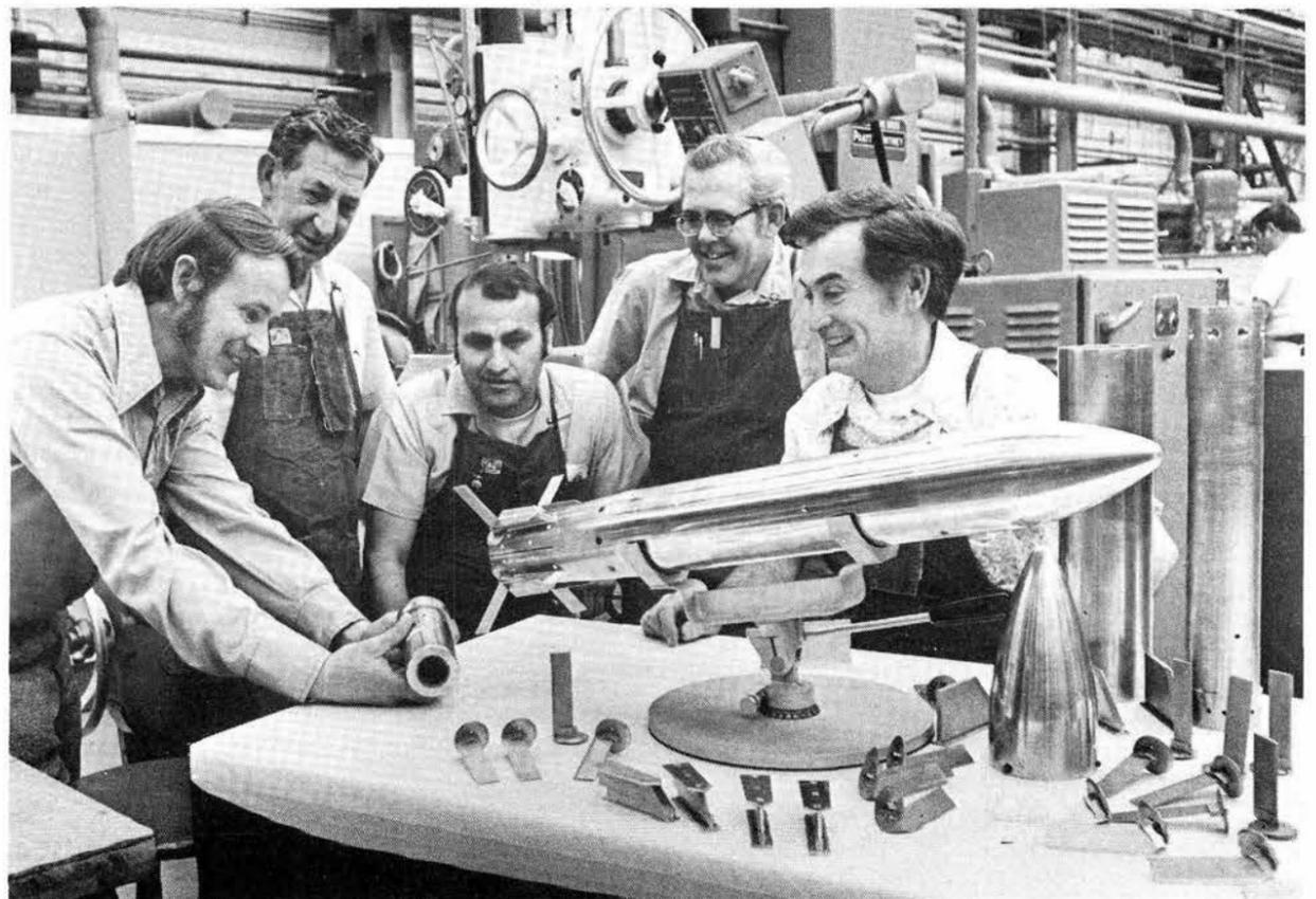
SCALE MODEL of weapon now under development was built for Structural Design Division 8157 for wind tunnel testing. It represents over 1500 hours of machining and is the work of (from left) design draftsman Bob Graham (8432) and machinists George Dawson, Andy Cardiel, Dell Houser and Bill Lavinsky of Machine Shop Section 8423-1. The intricate model has over 50 separate parts; Roger Everett is project engineer and Roger Page test engineer.
