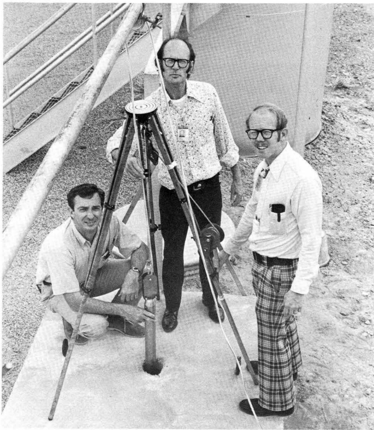
ABOUT TO lower neutron generator probe into test borehole are, from left, Ed Jacobs (2411), Gerry Smith and Lucien Rice (both 2442). Borehole is one of group of known uranium content at ERDA facility in Grand Junction, Colo. Pulsed neutron generator techniques have successfully characterized uranium content of various boreholes.
