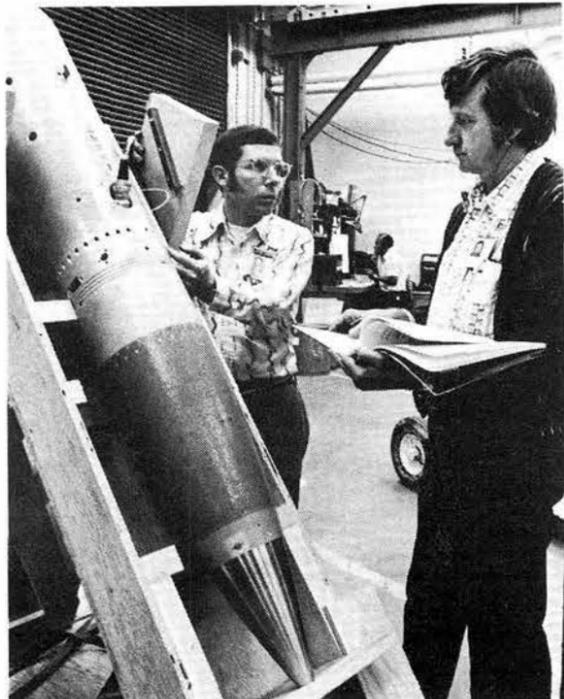
**MAGNETOMETER** in the nose section of a rocket launched from Cape Parry in the Arctic is checked by Hovey Corbin and Milt Zimmerman (both 1253) at Sandia prior to shipment. The magnetometer serves as a sensor for the rocket's guidance system to align the payload with the earth's magnetic field lines.
