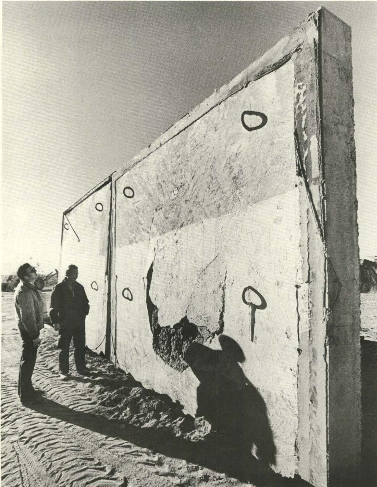
DAMAGE on back side of a 29,000 kilogram (32 ton) reinforced concrete slab after impact of 12-inch pipe is assessed by Al Stephenson and Jack Windsor. During impact tests, the slabs are grouted to a massive fully-instrumented frame.
