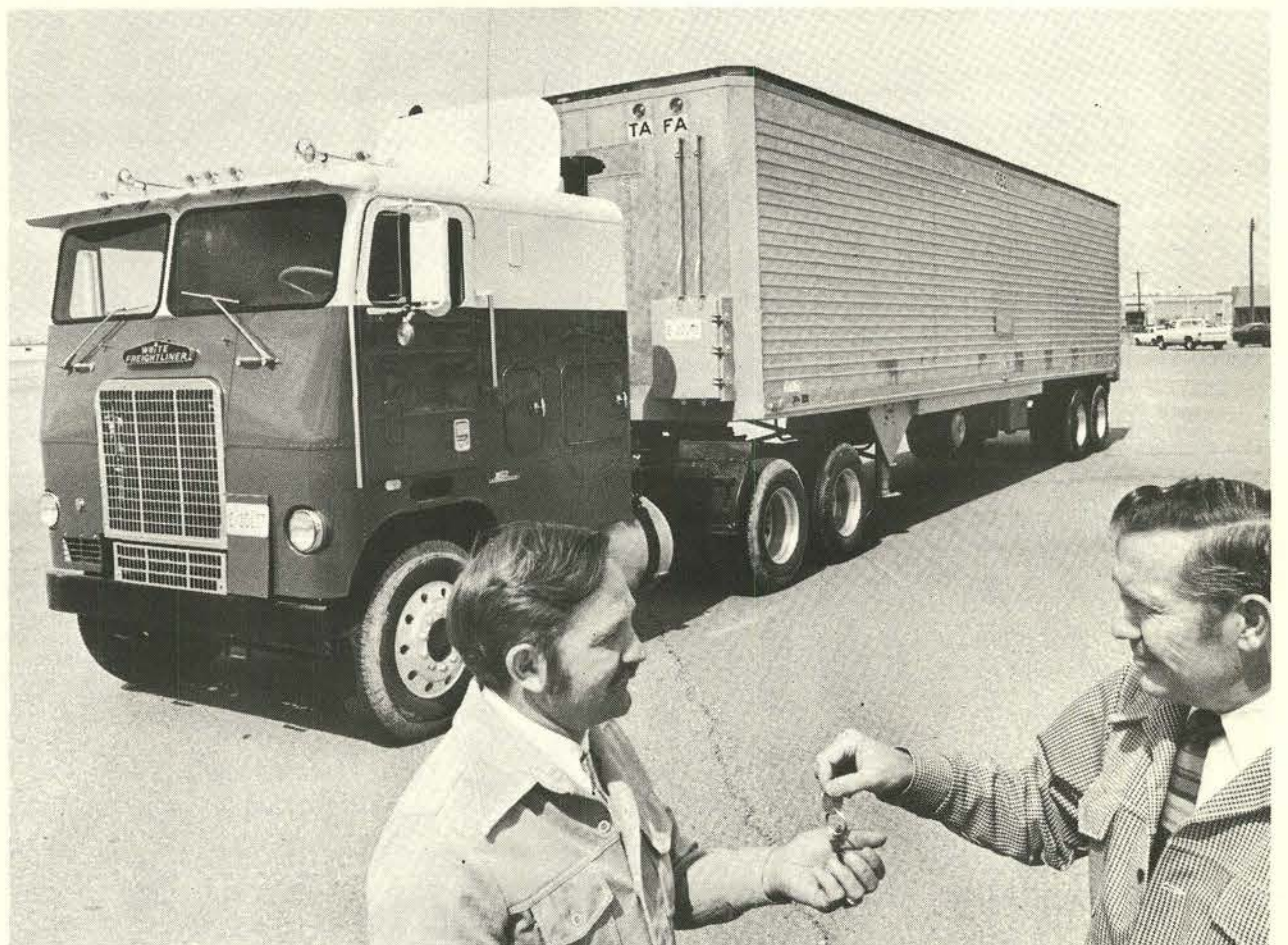
BERT VENDEL from ERDA's Transportation Safeguards Division kicked the tires, said "I'll take it," and Ed Bruce of Transportation Division 1714 hands him the keys. Trailer is special Safe Secure Trailer designed for ERDA/ALO in Ed's group for shipments of nuclear material, represents first of production run involving Rockwell Rocky Flats, Bendix Kansas City, and a number of commercial contractors. The big White tractor is also part of Safeguards' transportation program.
