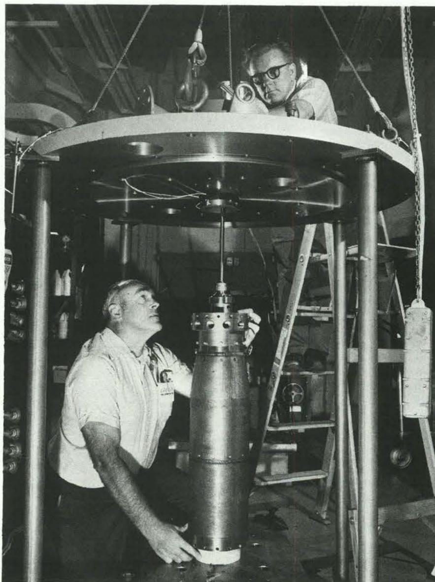
JOE BRADSHAW & HARRY OLSON (both 8413) adjust 8-inch test unit before high speed spin test.
