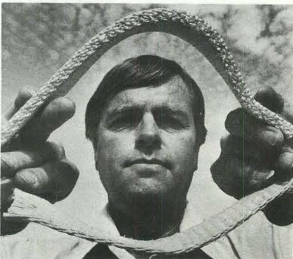
DRAMATIC DIFFERENCE in Kevlar and nylon is demonstrated by Bill Pepper (1332). Top nylon strap is twice as thick and heavy as bottom Kevlar strap. Both have a minimum breaking strength of 20,000 lbs.
