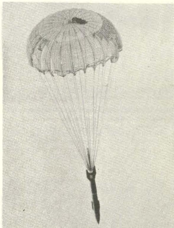
NEW PARACHUTE DESIGN for B61-3 has been undergoing testing at Sandia Laboratories. In this series of three photographs, the 24-foot-diameter parachute is subjected to a Mach 1.4 deployment and a load of 90,000 pounds at Sandia’s rocket sled facility. New material, Kevlar-29, is used in the chute. The project is centered in Parachute Systems Division 1332 under Dave McVey.
