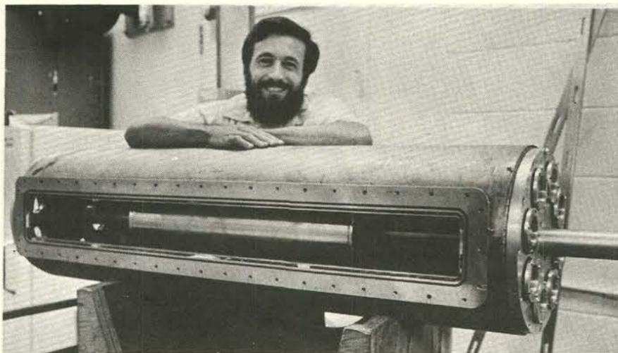
PAUL BOLDUC (5232) displays his cylindrical electron beam diode device recently patented by ERDA.
