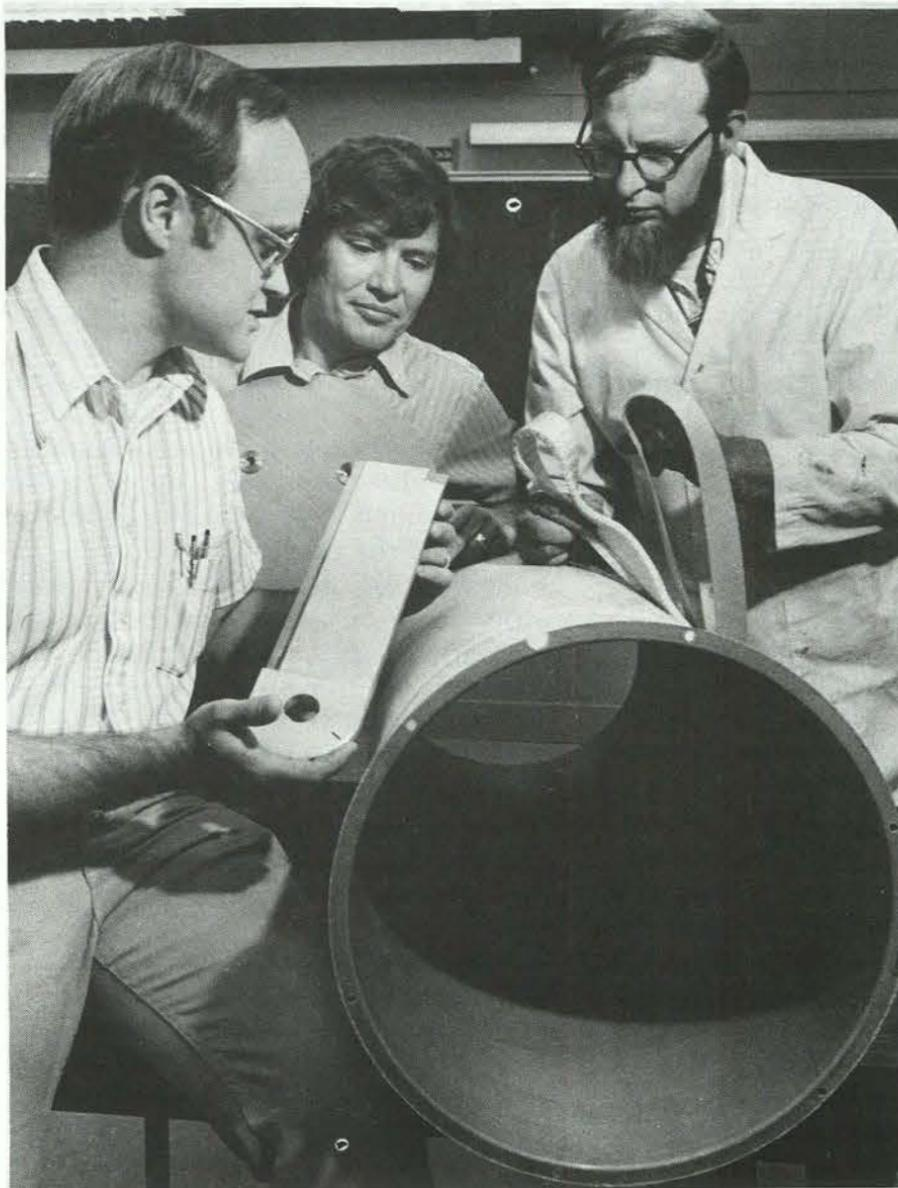
**MATERIALLY DIFFERENT.** That's what these B77 parts are. Left to right, Bill Hoover holds a boron-aluminum fin; Ron Allred clutches the weapon's aft cover and leans on the parachute liner (both are Kevlar-epoxy laminates); and Dick Ericksen demonstrates the difference in thickness between a nylon chute webbing strap (his right hand) and (in his left) a Kevlar strap of the same strength.
