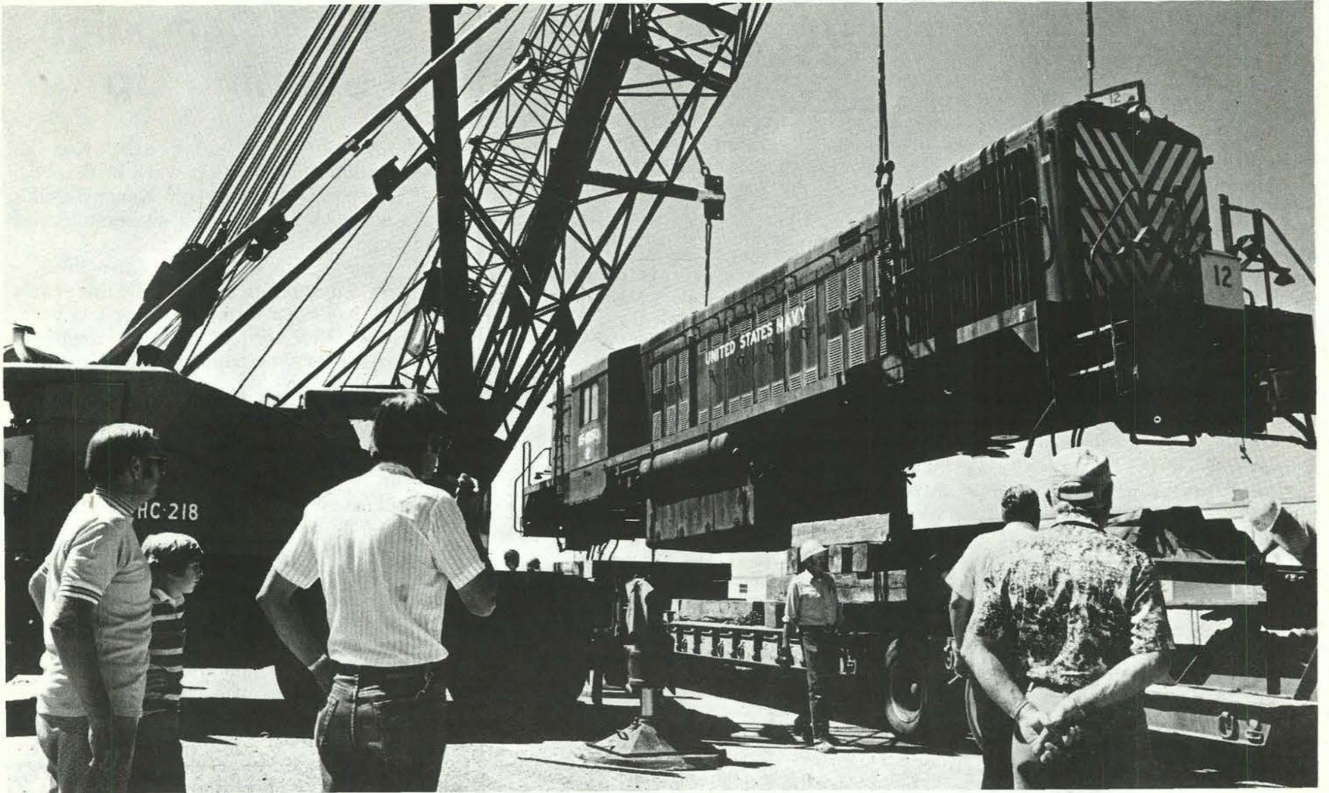
**SURPLUS** locomotive, scheduled for a spectacular demise in Area III in January or February, is lifted onto a flatbed truck for transport. The unit, sans wheels (or trucks as they're called), weighs 125 tons. It will be propelled by rockets at 80 mph down Sandia's sled track to impact into a truck containing a shipping cask with simulated waste nuclear fuel. Test will measure the cask's integrity under "worst kind" of
