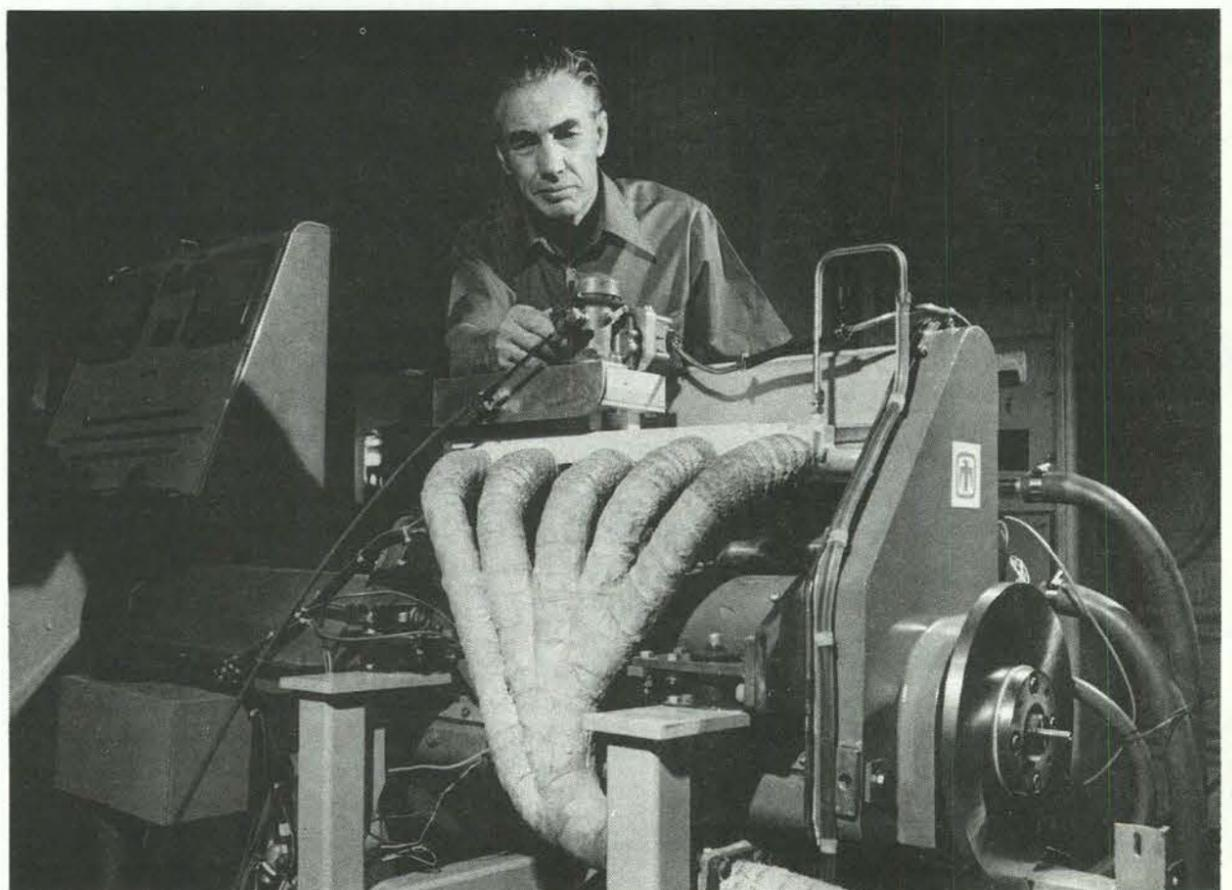
THE MAN AND THE ENGINE — Inventor Harvey Pouliot and variable displacement engine that offers significant fuel economy. Harvey is a member of Sandia Livermore's Combustion Applications Division (8116).
