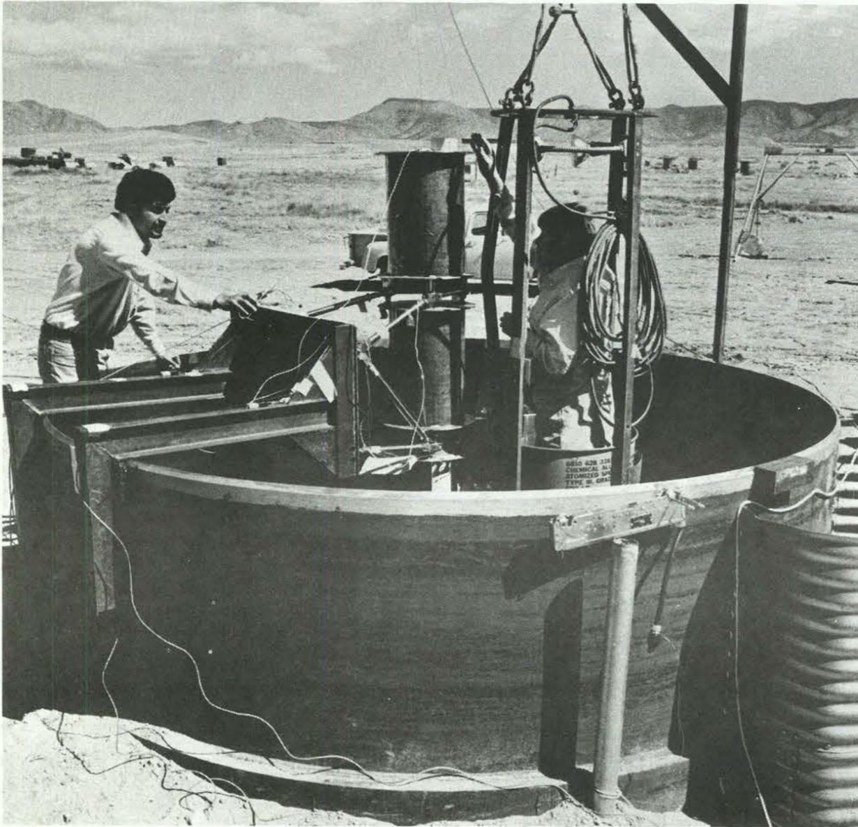
VERTICAL SHOCK TUBE in Coyote Test Field is readied for a test of space RTG units. Manny Vigil and Tom Witherspoon (both 9335) install instrumentation. Tube is 6 metres long; 7½ kilograms of HE was detonated at the bottom of pipe to simulate a launch pad explosion.
