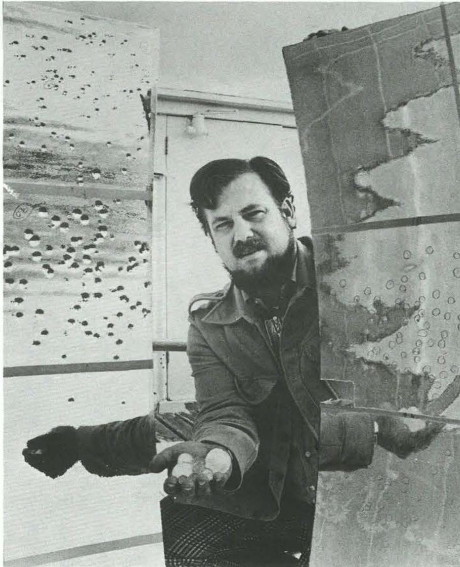
**TEST RESULTS:** Barry Butler (5844) holds ice balls — up to 4 cm in diameter — used in environmental tests of parabolic solar reflectors. Aluminum-skin, aluminum-honeycomb core sandwich reflector at left shows extensive damage from the hail-simulation test, while the fiberglass-skin and core reflector at right suffered much less damage (impact points circled in order to be readily noticeable).
